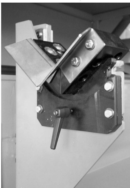
Fig. 3.4 -6 Vee fitted with ball bearings for circular tubes
