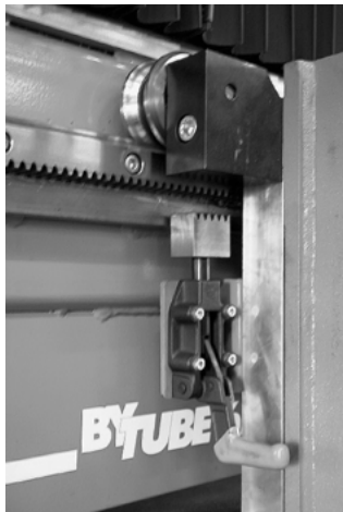
Fig. 3.5 -5 Tailstock
