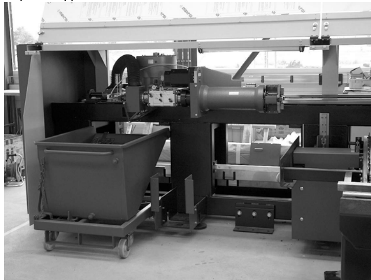
Fig.3.4-14 Emptying the small parts hopper
