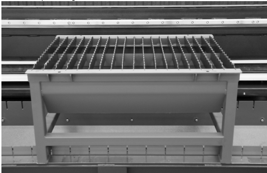
Fig.3.5-19 Table for flat-part cutting
