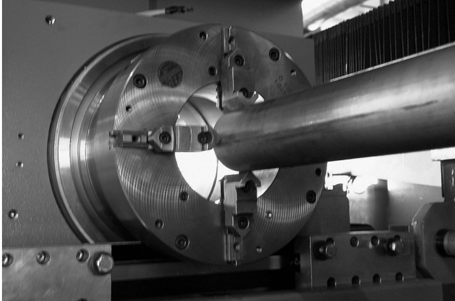
Fig. 3.5 -4 Manual loading with four-jaw chuck and tailstock
