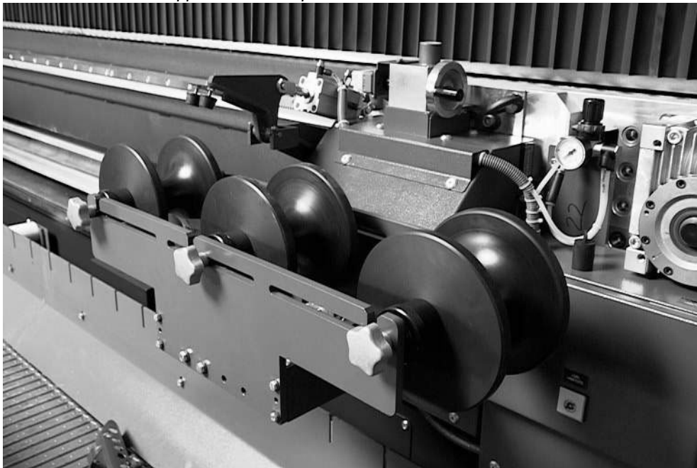
Fig.3.5-16 Travel unit with tube support for tubular profiles
