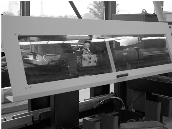
Fig. 3.2 -2 Tube loader safety cover with safety sensor
