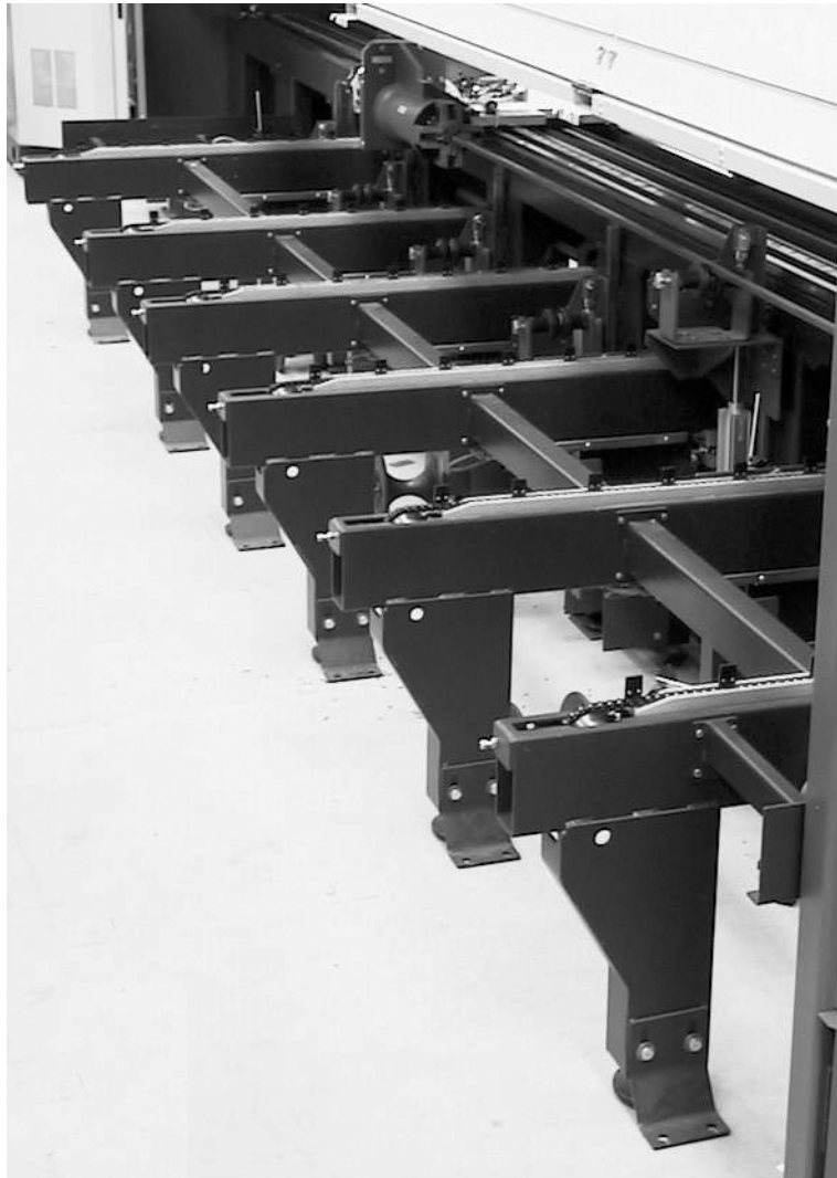
Fig. 3.4 -2 The tube magazine can hold 6 or 12 tubes.
