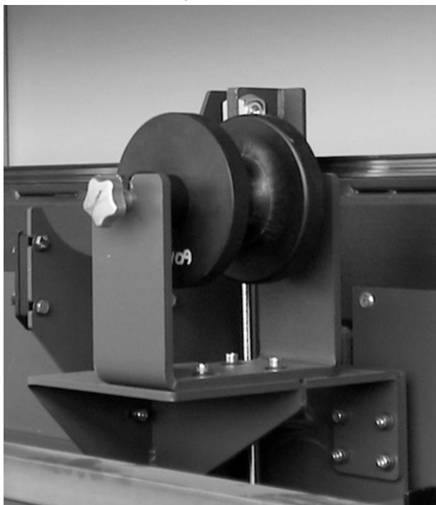
Fig. 3.4 -5 Support roller for rectangular tubes
