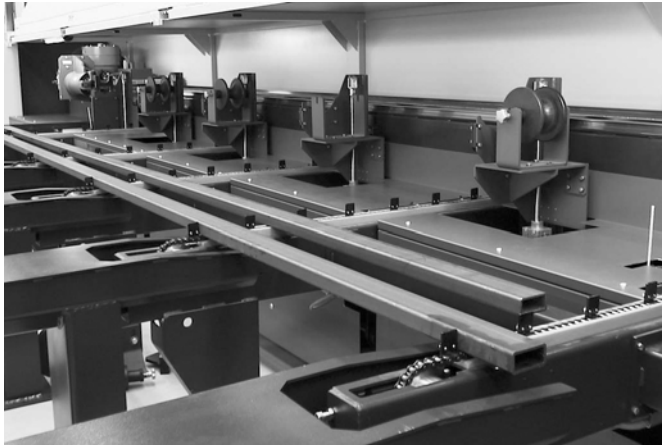
Fig. 3.4 -3 Tube loader with raised pillar rests
