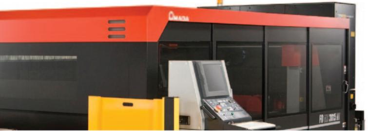
The FOM2 incorporates a rack and pinion drive system in the X-axis and high-precision ball screws in the Y and Z-axis. For over ten years, the FO series has established and earned a worldwide reputation for unparalleled accuracy and reliability. As the latest generation, the FOM2 series continues to set new standards for precision and performance.
