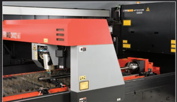
Providing for quick and efficient processing of round and square tubing, an optional rotary axis further enhances the capabilities of the FOM2.
