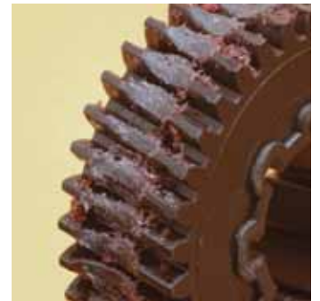
Figure 28 Tooth deformation due to excessive heat
