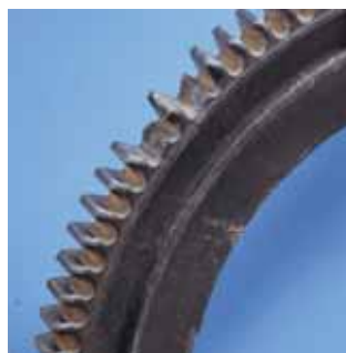
Figure 29 Tooth fracture at root due to over loading
