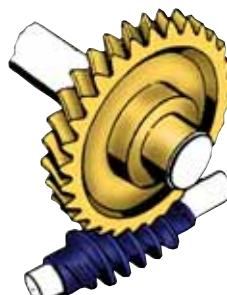
Figure 8 Single Enveloping Worm Gear
