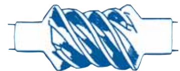
Figure 9 Double Enveloping Worm Gear
