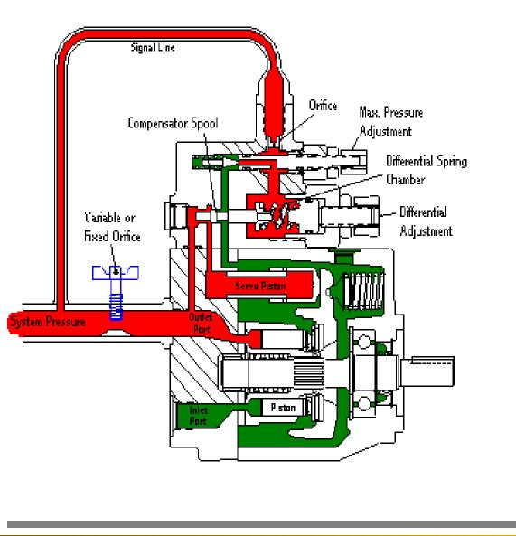
Since the load sense control will adjust pump flow to maintain the pressure drop across the orifice constant, increasing the orifice size will increase the flow to the system. Closing the orifice , will decrease the flow to the system.
