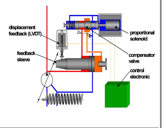
A proportional displacement control will position the swashplate angle proportional to a input voltage signal to the solenoid. The output flow can be adjusted, without affect from system pressure. A LVDT feedback signal of the swashplate angle closes the loop electronically. An amplifier card in the electronic controller compares the command signal and the feedback signal and sends a voltage signal to the proportional solenoid to position the swashplate.
