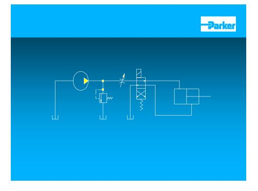
(HP = GPM \* PSI | 1714 assume 100 % efficiency)
