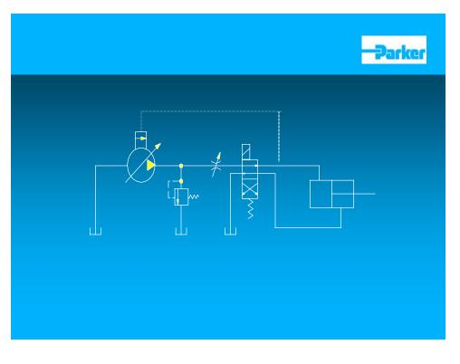
(HP = GPM \* PSI | 1714 assume 100 % efficiency)
