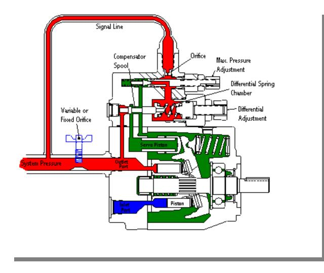
In this view the variable orifice is wide open and it is not restricting the pump flow. Pump outlet pressure and load pressure are equal. Since the pressure is equal on both sides of the spool, the differential spring keeps the spool to the left. There is no control pressure in the servo piston, so the pump will stay at full stroke.
