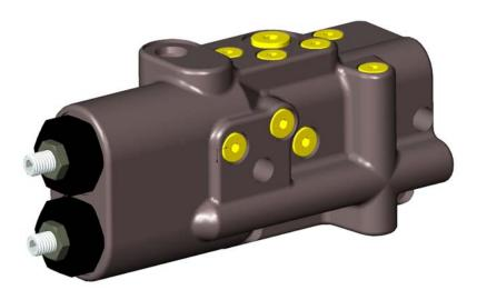
Piston Pump Controls are integral valves that port flow to a stroking piston in response to a pressure or electronic signal, which results in a variable hydraulic pump achieving a desired displacement.
