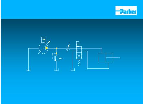
Remember the Fixed Pump system used 17.5 HP and wasted 11.6 HP
