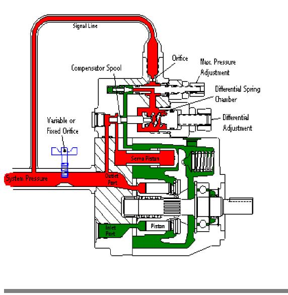
Increasing the pump drive speed will increase the pump output flow , but since the load sense control is working to maintain a constant pressure drop across the orifice, the load sense pump will destroke to maintain the same output flow.
