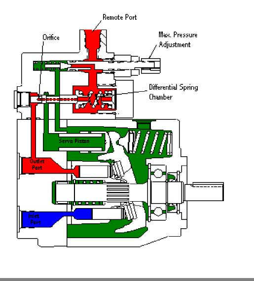
Just like a standard Pressure Compensator, except the pressure limiter adjustment is done with an external relief valve.
