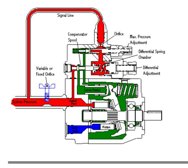
A load sense compensator will react to increases in the load by increasing output pressure. This is done by sensing the pressure drop across an external orifice and adjusting displacement to maintain a constant pressure drop across the orifice.
