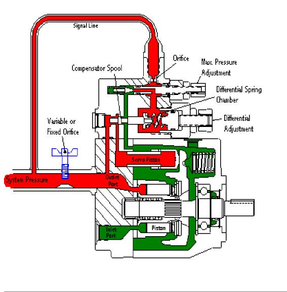
In this view the variable orifice is restricting pump flow. Pump outlet pressure is increased and a pressure drop is created across the orifice. The pump pressure will increase until it overcomes the differential spring force and shifts the spool to direct control oil into the servo piston and destroke the pump. The pump will maintain a flow level that keeps the pressure drop across the variable orifice constant ( equivalent to the differential spring setting).
