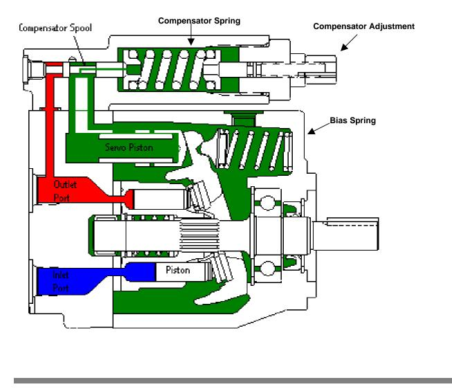
Pump Pressure is below setting of control Pump is at Full Stroke
