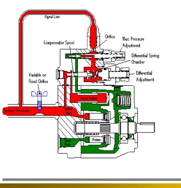
If the load pressure increases, the pump outlet pressure will increase proportionately to maintain the constant pressure drop across the orifice.
