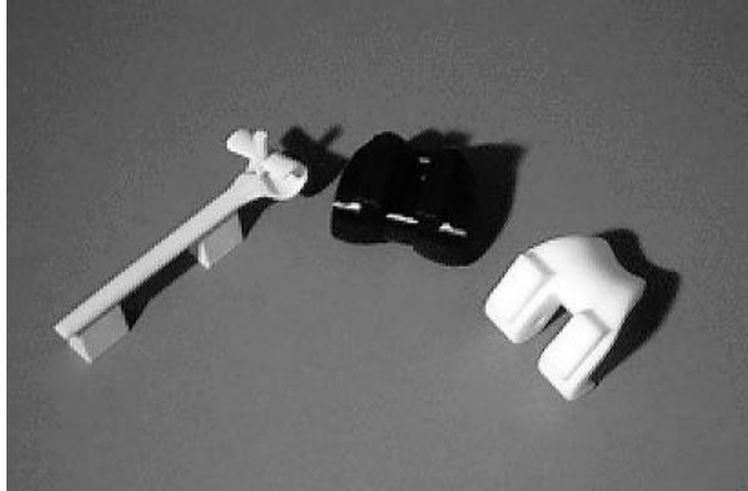
Photo 5. ABS IC pattern for an elbow (with gating) and two knees (Biomet).
