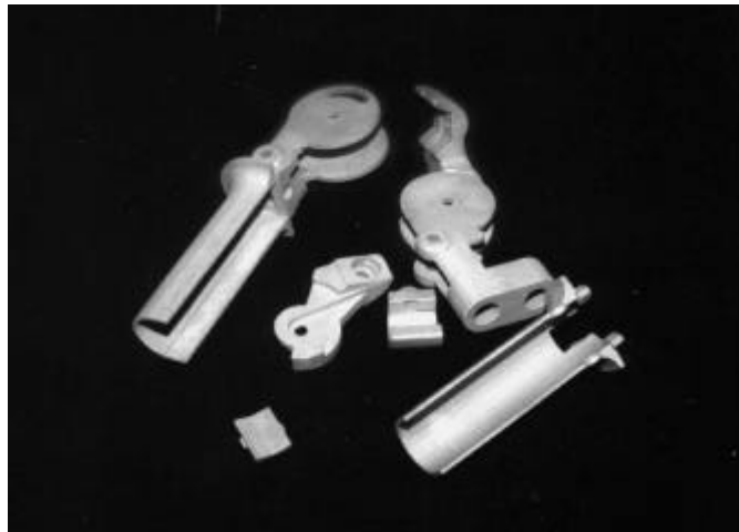
Photo 8. Aluminum Investment Castings from ABS Patterns (Quebec Hydro)
