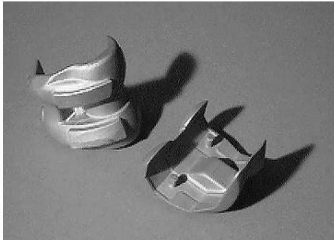
Photo 6. Example of two cobalt chrome knee implant investment castings (Biomet).
