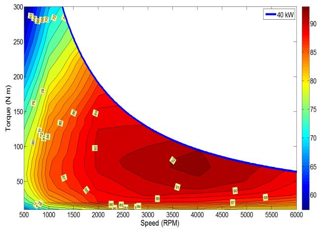
Motor/Inverter Efficiencies at 500VDC
