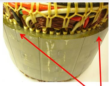
Stator laminations are made from separate pieces
