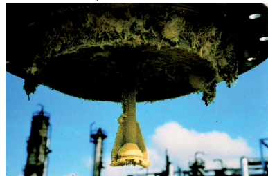
Figure 2: A Rosemount parabolic antenna coated in sulfur.
