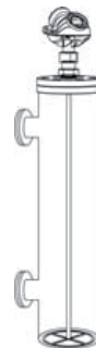
A centering disk helps to keep the probe away from the chamber walls. It is recommended for single rigid probes. Its applicability with long flexible probes is more limited.
