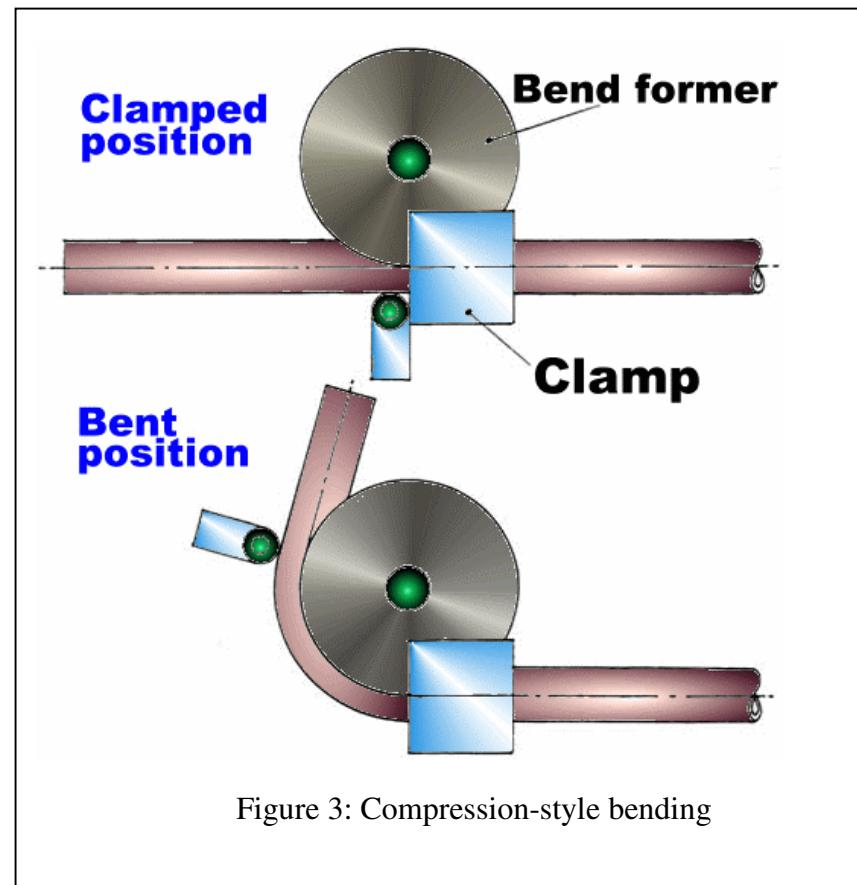
Figure 3: Compression-style bending
