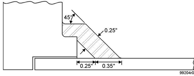
Figure 3. Weld Overlay Design
