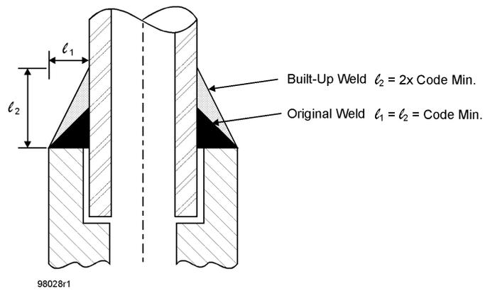
Figure 2. 1 x 1 Weld Built Up to 2 x 1
