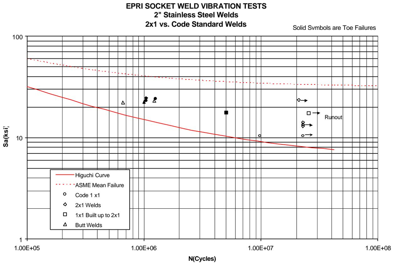
Figure 4. Weld Size, Stainless Steel
