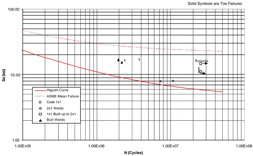
Figure 5. Weld Size, Carbon Steel
