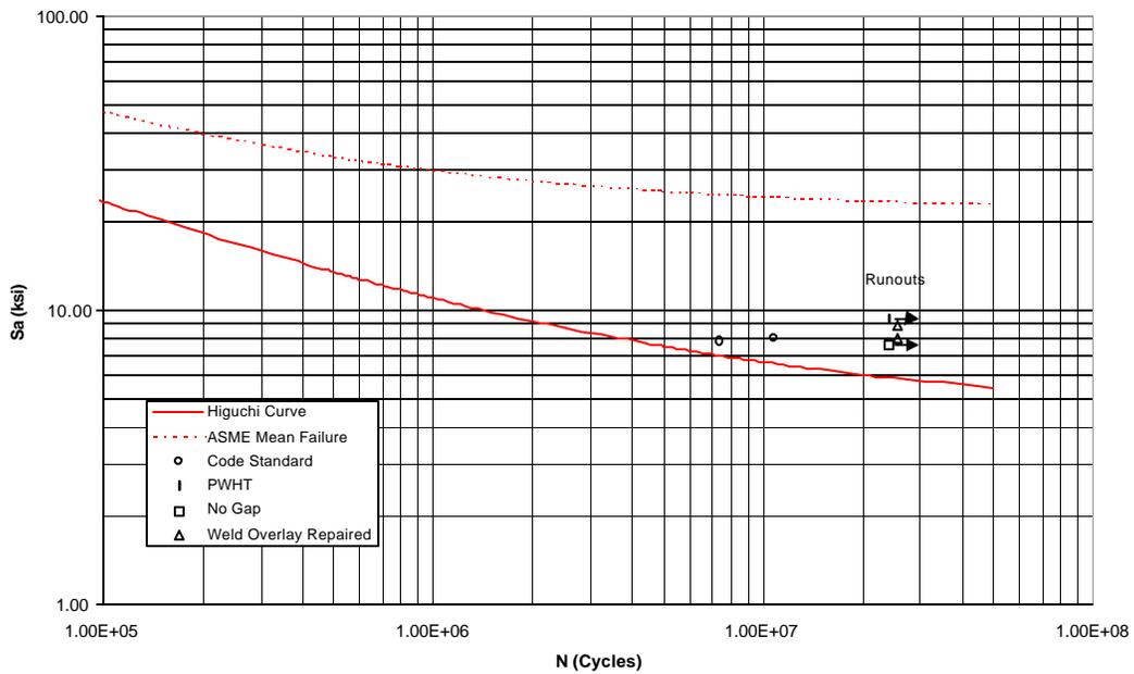
Figure 8. Weld Enhancements, Carbon Steel
