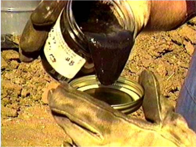
Figure 5 Sidestream sample from passing gel pig fluid, with a considerable quantity of black powder in suspension.
