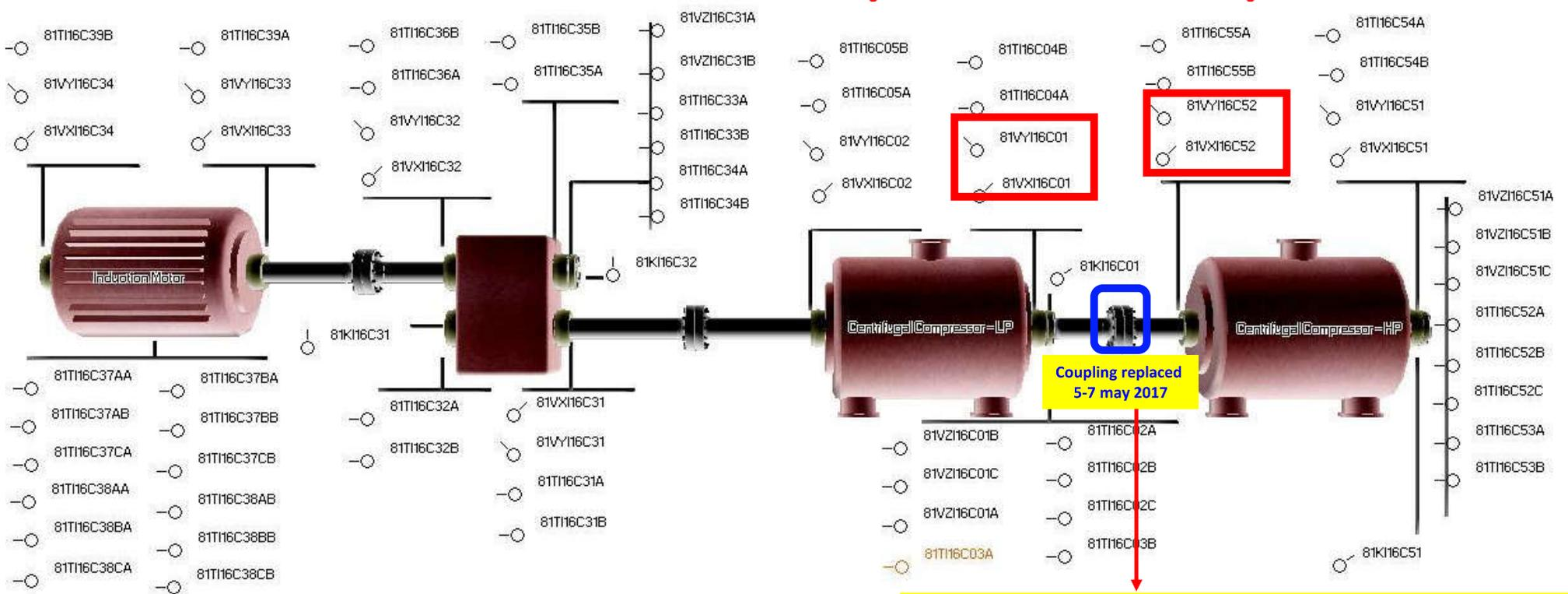
Based on previous failure pattern, the present data indicates, change in the coupling balance condition and most probably by breaking of the shim pack elements.
