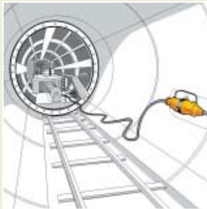
A tunnelling application for power feed to a full-face drilling machine.
