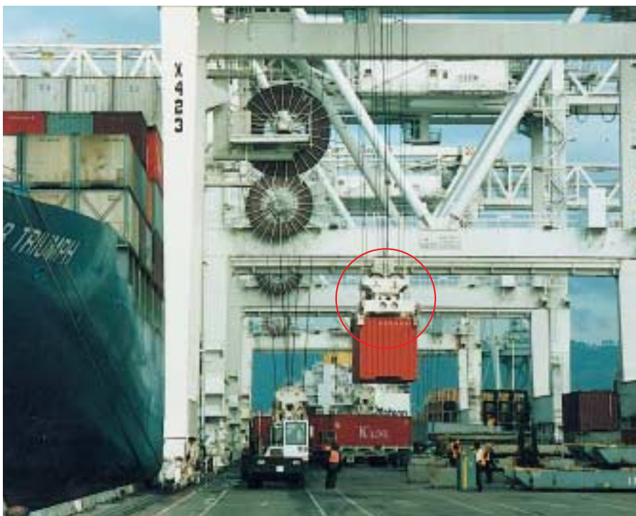
Plugs & Sockets of Push & Pull type are used to connect quickly and easily on various crane equipment like spreaders, vacuum-loaders, hydraulic grabs and other crane lifting equipment.
