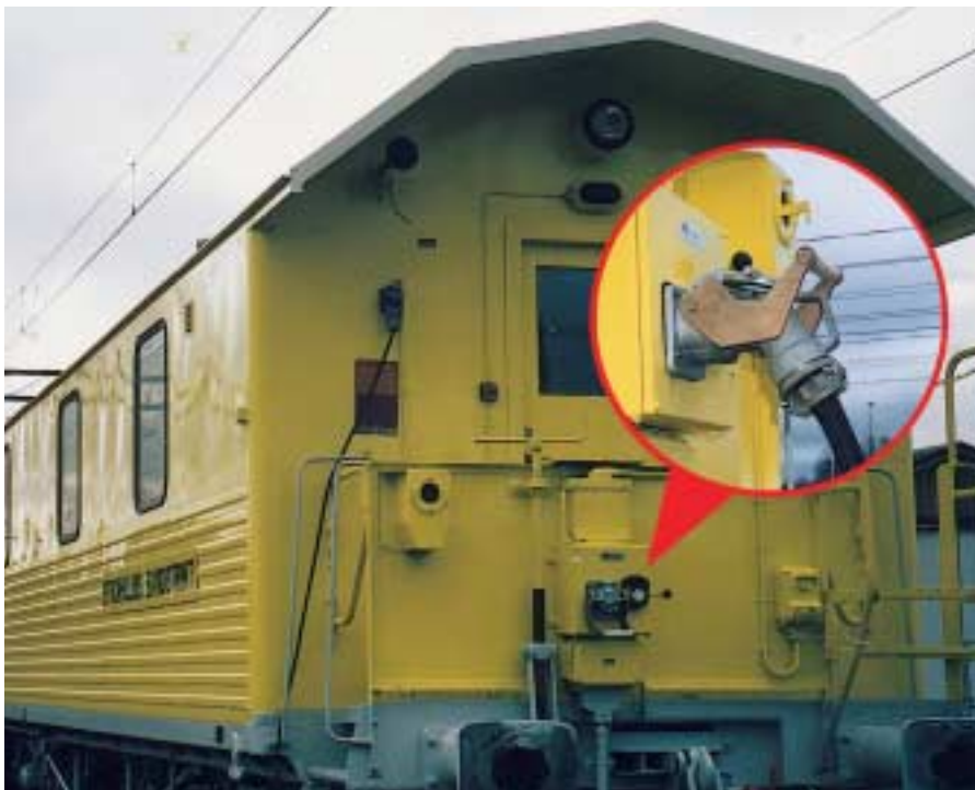
The above photo shows a typical connector application on a ballast service wagon of the Swedish Railways (Banverket).
