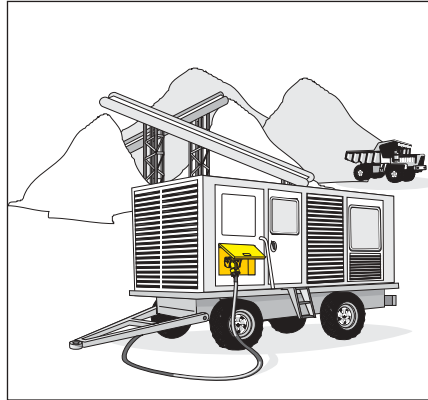
Electrical connectors are used for mobile generator sets for telecommunication networks, open pit mines and other major users of electrical power.
