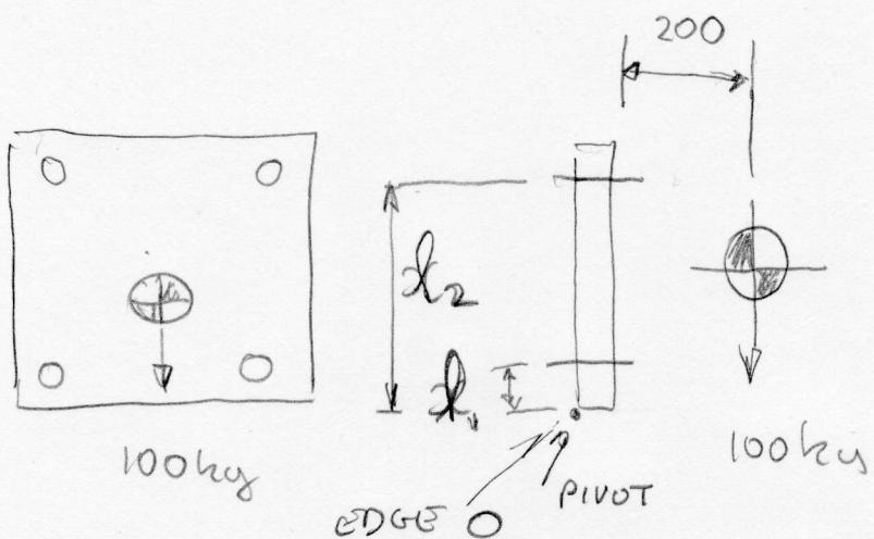
SHEAR IN BOLTS  $\frac{9.81 \times 100 \text{ kg}}{4} = 245.25 \text{ N}$
