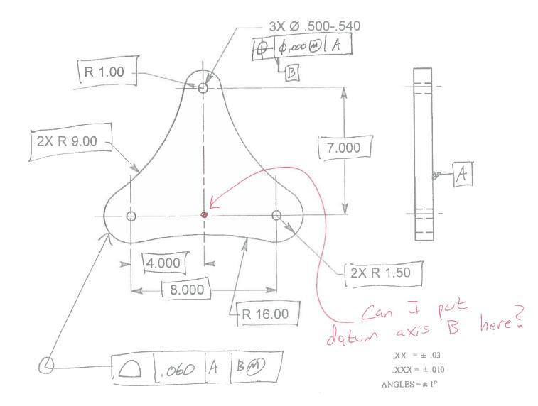
39. The hole pattern is for ½-inch fasteners. Locate the three holes to each other and perpendicular to the back of the part within the required tolerance. Next specify a profile tolerance perpendicular to the back of the part and located to the hole pattern within .060. Complete the drawing using MMC/MMB wherever possible.
