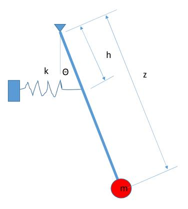
A beam is acting as a pendulum, with a mass concentrated on the end. There is a spring attached to the beam. Need to develop a relationship to estimate the maximum bending moment that occurs in the beam when the system is vibrating at it's natural frequency. Assume that the beam has no mass, that has been considered in the effect "m" at the end of the pendulum. The beam is NOT rigid. Small angle assumption can be made.
