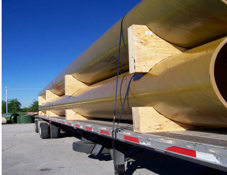
Figure 7-2 Typical Wooden Cradle Supports and Tie Down for Large Diameter Pipe Transport; ( Photograph courtesy of Fiber Glass Systems and Fiberglass Solutions Inc )
