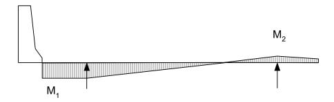
Figure 2-12 Assumed Distribution of the Collision Moment Across the Width of the Deck
