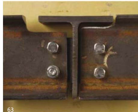
Fig. 3.5A Joint gap minimized. The gaps on the left are standard structural steel, and on the right sized for AEES. (Courtesy of AISC)
