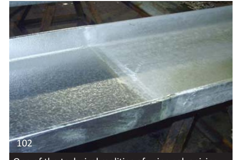
102 One of the technical realities of using galvanizing as a finish lies in the inconsistency of the product. The difference in this photo is due to finishing temperatures. If galvanizing is used as a final coating on an AESS project, differentials in finish must be both understood and detailed into the project.
