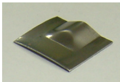
Fig 2: Complex formed Flat Spring geometry
