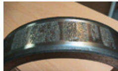
Fig 7d – Damage in Inner Raceway was confirmed.
