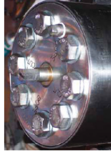
AutoShift cartridge with center manual shift extension
