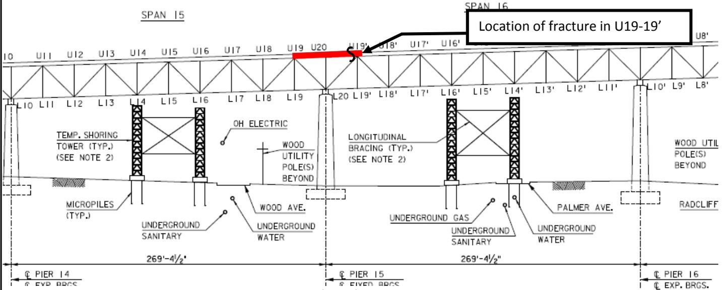
Figure 5 Shoring Tower locations, elevation looking north (HNTB)
