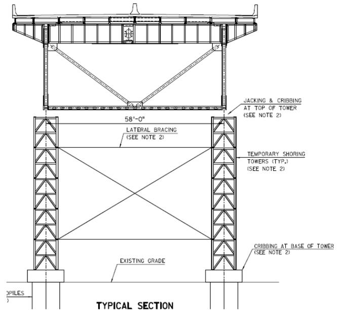
Figure 6 Shoring Tower typical section, looking east
