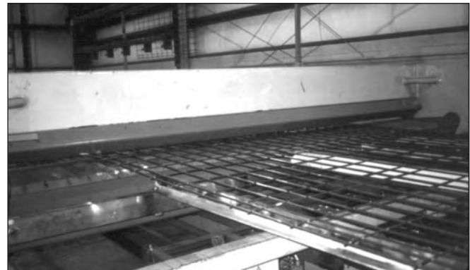
Latest WWR machinery can weld to 3/4" diameter wires.
