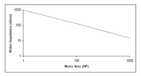
Figure 2. Motor impedance relative to motor size
