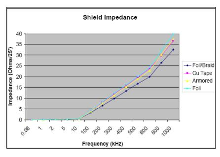
Figure 4. Shield/Ground impedance of the various cable types
