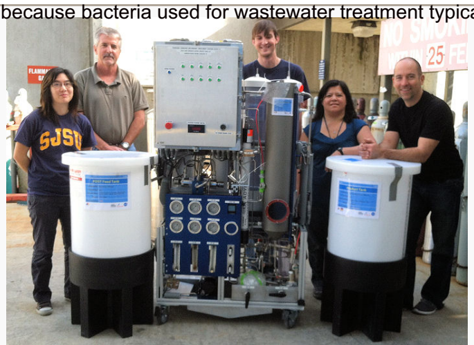
Flynn (second from left) and other researchers stand next to a forward osmosis water recycling system, a membrane-based passive wastewater treatment system. Photo courtesy of Flynn, NASA.
