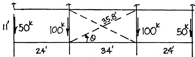
Type 2 Construction - simple framing,  $F_y = 36 \text{ ksi}$
