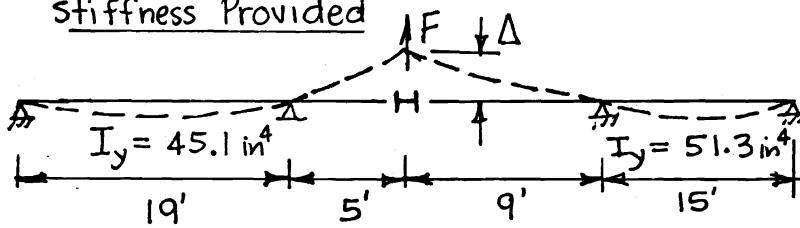
$$\frac{\Delta}{L} = \frac{F_a^2(a+b)}{3EI} \quad (\text{AISC Manual}) \quad \beta = \frac{F}{\Delta} = \frac{3EI}{a^2(a+b)}$$
