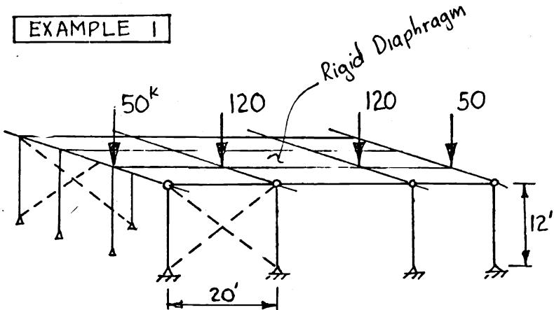
REQ'D: SIZE OF TENSION BRACES TO STABILIZE THE SYSTEM
