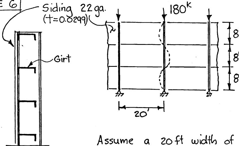
Is the 22ga. siding sufficient to support the girts so that the columns are braced at the one-third points? Siding is attached to the girts in a standard manner using screws for fasteners.
