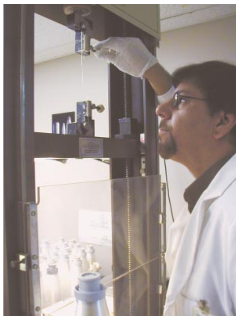
Tensile strength test performed on Quartzel®
