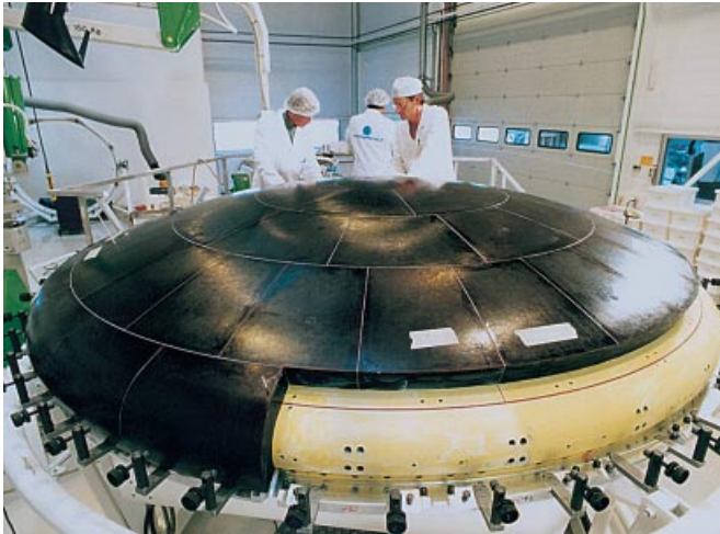
Atmospheric Reentry Demonstrator heat shield. This resin impregnated Quartzel® fabric withstands temperatures of 2 000°C reached during reentry due to atmospheric friction.
