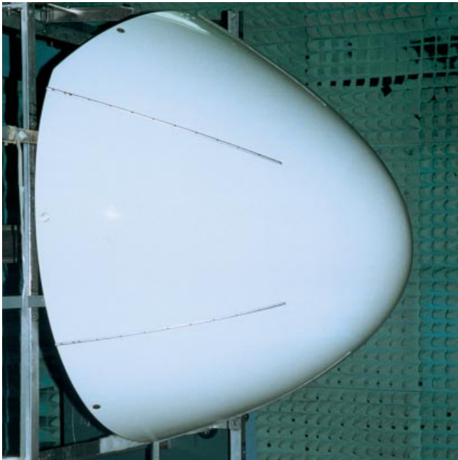
Boeing 757 radome under test at Saint-Gobain Performance Plastics
