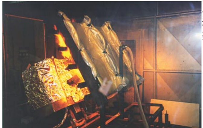
Quartzel® fuselage fire barrier under test at C.E.A.T. (Toulouse – France)
