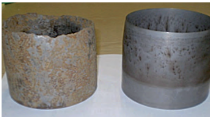
A deformed (left) and new (right) Archway UT100 cutting shoe provided by BAM Ritchies
