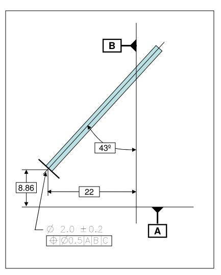
Common... Detailing coordinates at one end of an angled hole and typically disregarding control of the spot face surface
