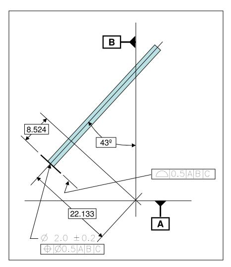
Better... Detailing basics that are required to inspect the feature position and spot face surface profile "if necessary".
