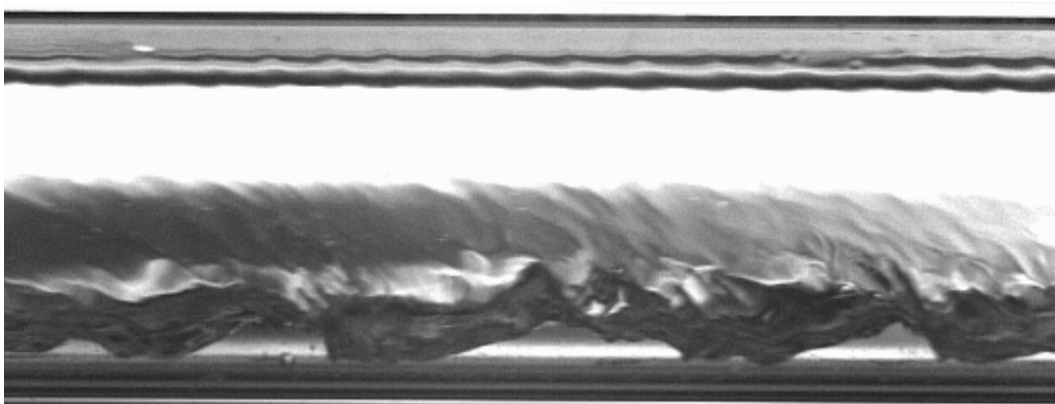
Figure 32: Still image from high-speed video of R134a with a bulk enthalpy of 388 \text{ kJ kg}^{-1} ( x=0.77 )
