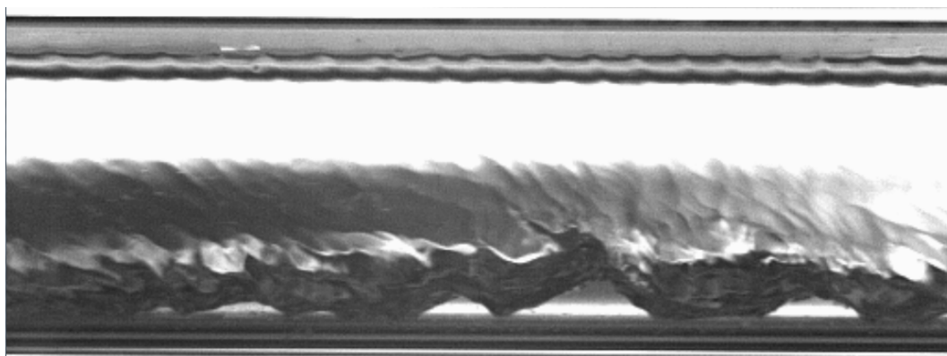
Figure 30: Still image from high-speed video of R134a with a bulk enthalpy of 402 \text{ kJ kg}^{-1} ( x=0.86 )
