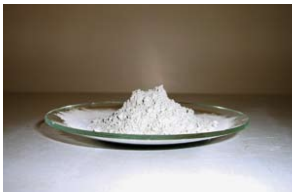
Figure 6 Low alkali cement reduces the risk of efflorescence
