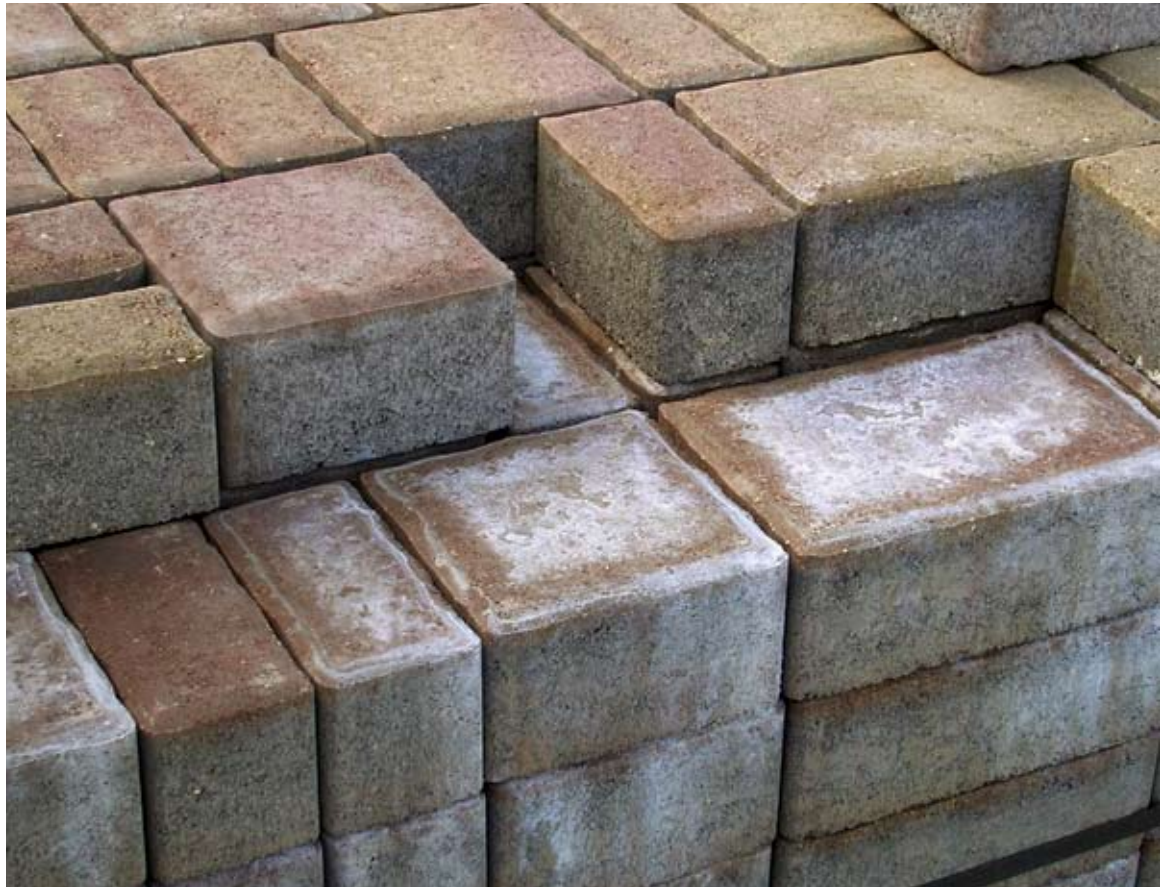
Figure 1 Concrete paving stones with efflorescence stains after stocking outdoor
