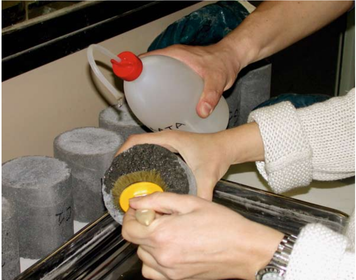
Figure 10 Chemical or mechanical removal of efflorescence should be conducted carefully to avoid surface damage.
