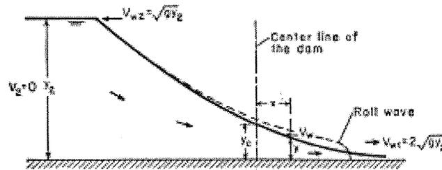
FIG. 19-10. Wave profile due to dam failure.
