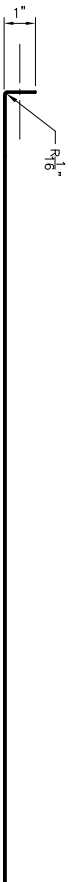
211A INERTIAL SEPARATOR POCKET END SIXTY (60) REQ'D. FAB'D FROM 304 SS. 18 GA. X 11 3/16" X 26 5/16"
