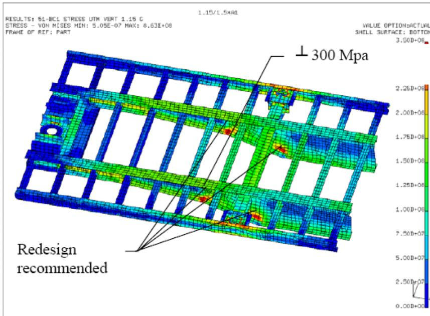
Results (von Mises stresses in Pa) for the vertical fatigue load case, front part of trailer seen from above.
