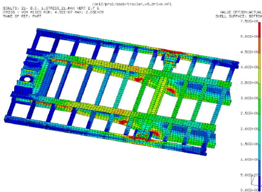
Results (von Mises stresses in Pa) for the vertical load case.
