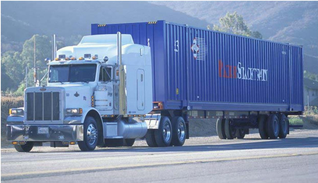
**Figure 12, 53 feet container for freight transport**
