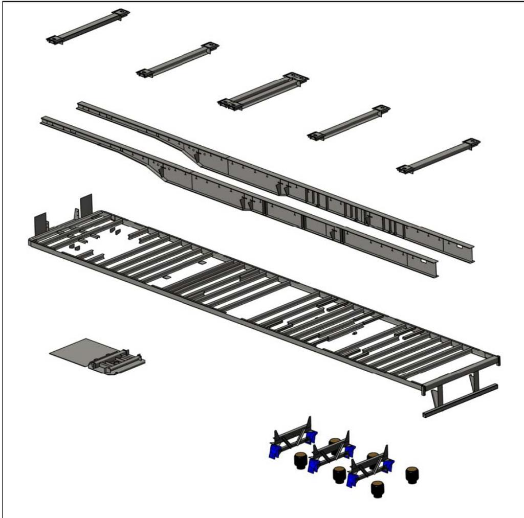
**Figure 20. Trailer chassis assembly**
