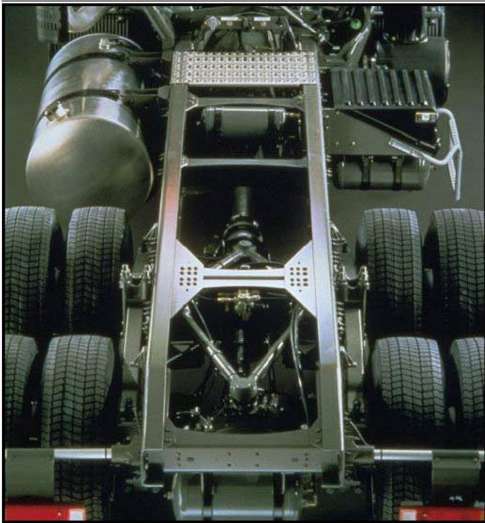
**Figure 14, Truck frame rails in extra high strength steel**
