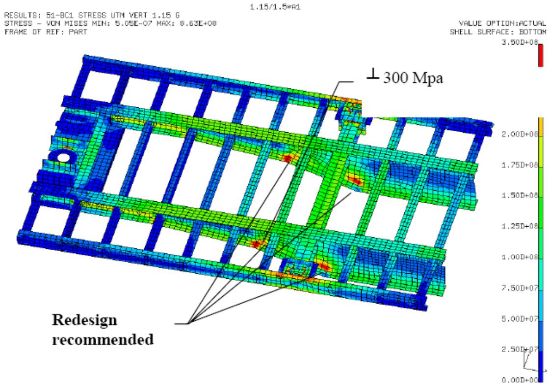
Figure 25. Von Mises stresses over max. Vertical fatigue loadcase
