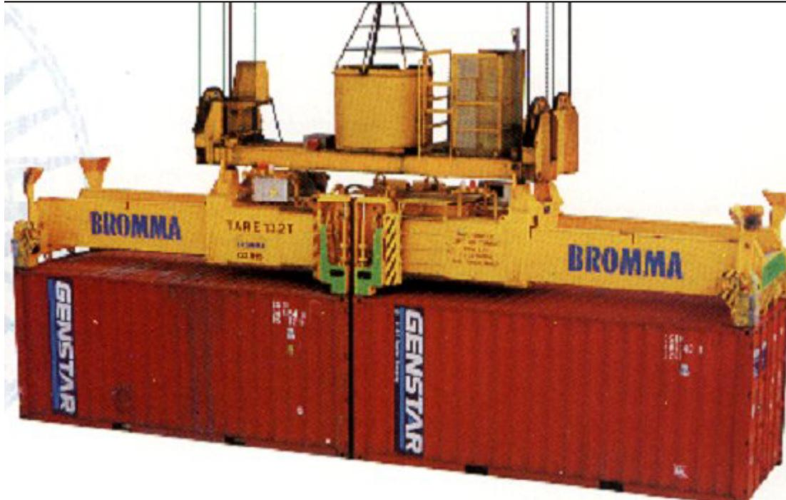
Figure 11, Container spreader
