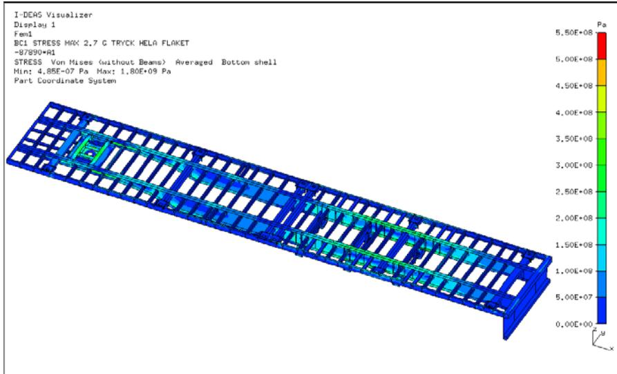
**Results (von Mises stresses in Pa) for the distributed maximum load case.**
