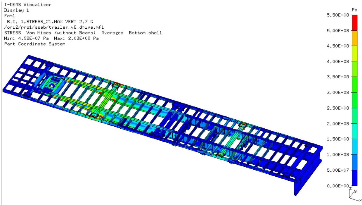
**Figure 23. Von Mises stresses over max. vertical static loadcase**
