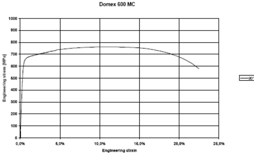
**Figure 5, Typical stress strain curve for Domex 600 MC**
