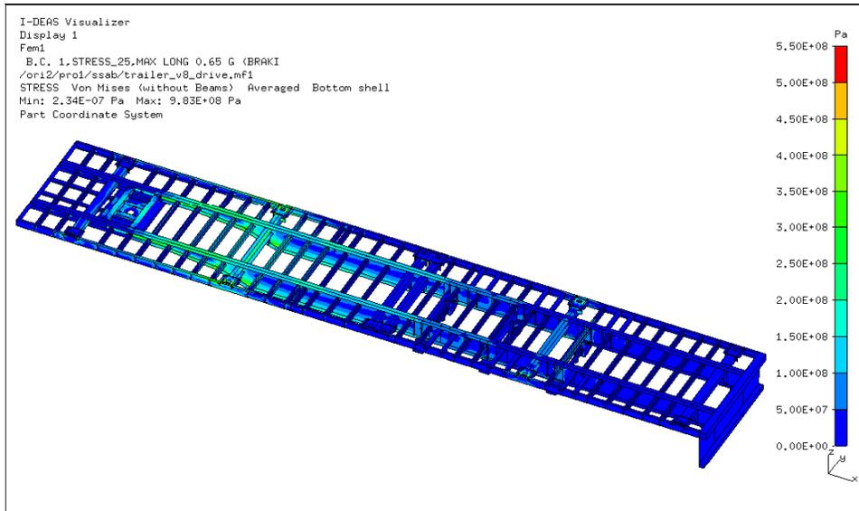
Results (von Mises stresses in Pa) for the longitudinal maximum load case.
