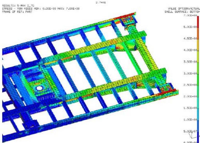
**Figure 26. Von Mises stresses over max. Vertical static loadcase with stiffeners added.**
