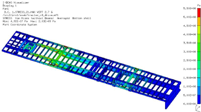
Results (von Mises stresses in Pa) for the vertical load case.
