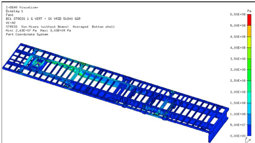
Results (von Mises stresses in Pa) for the torsion maximum load case.
