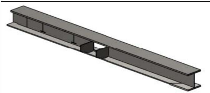
Figure 29. Section A of side member
