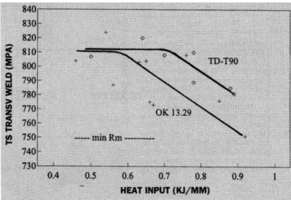
Figure 6, Tensile strength of MAG welded joints. One matching electrode OK 13.29 (tensile strength 820 MPa) was used.
