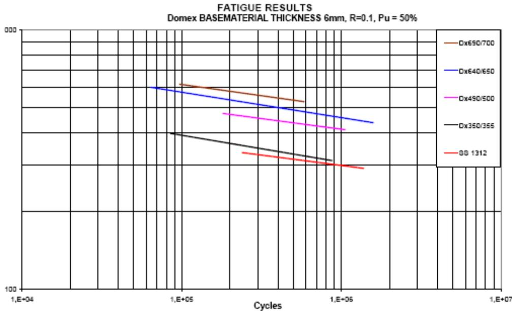
Figure 22. S-N diagram for Domex steels
