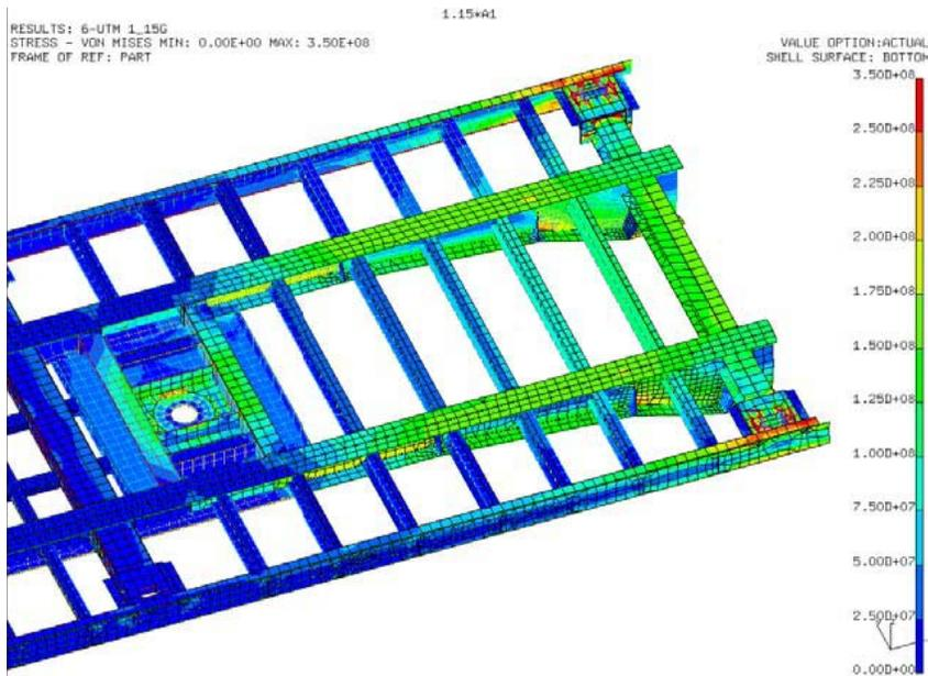
**Figure 27. Von Mises stresses over max. Vertical fatigue loadcase with stiffeners added.**
