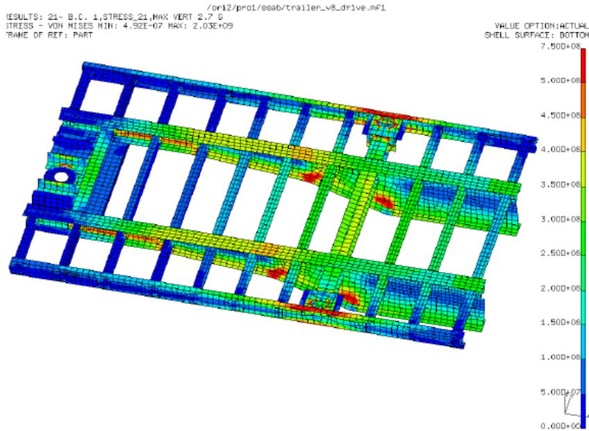
Results (von Mises stresses in Pa) for the lateral maximum load case.
