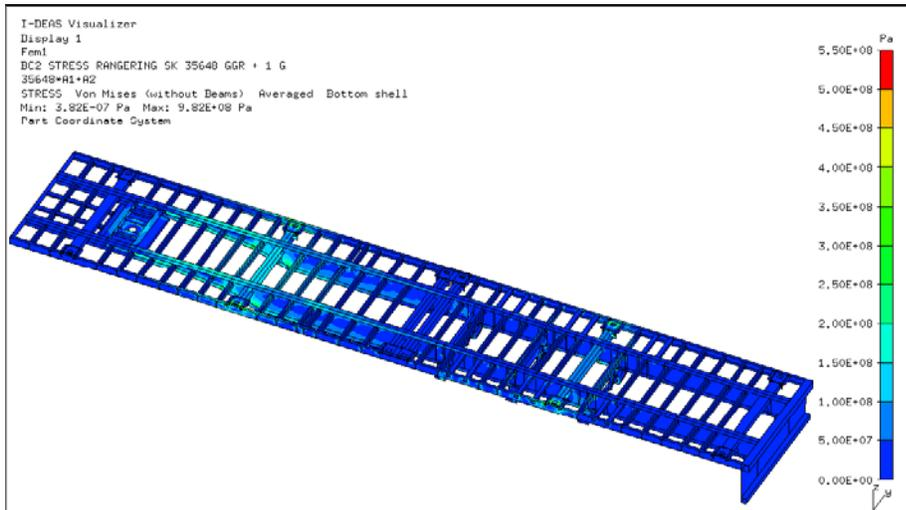
Results (von Mises stresses in Pa) for the marshalling maximum load case.
