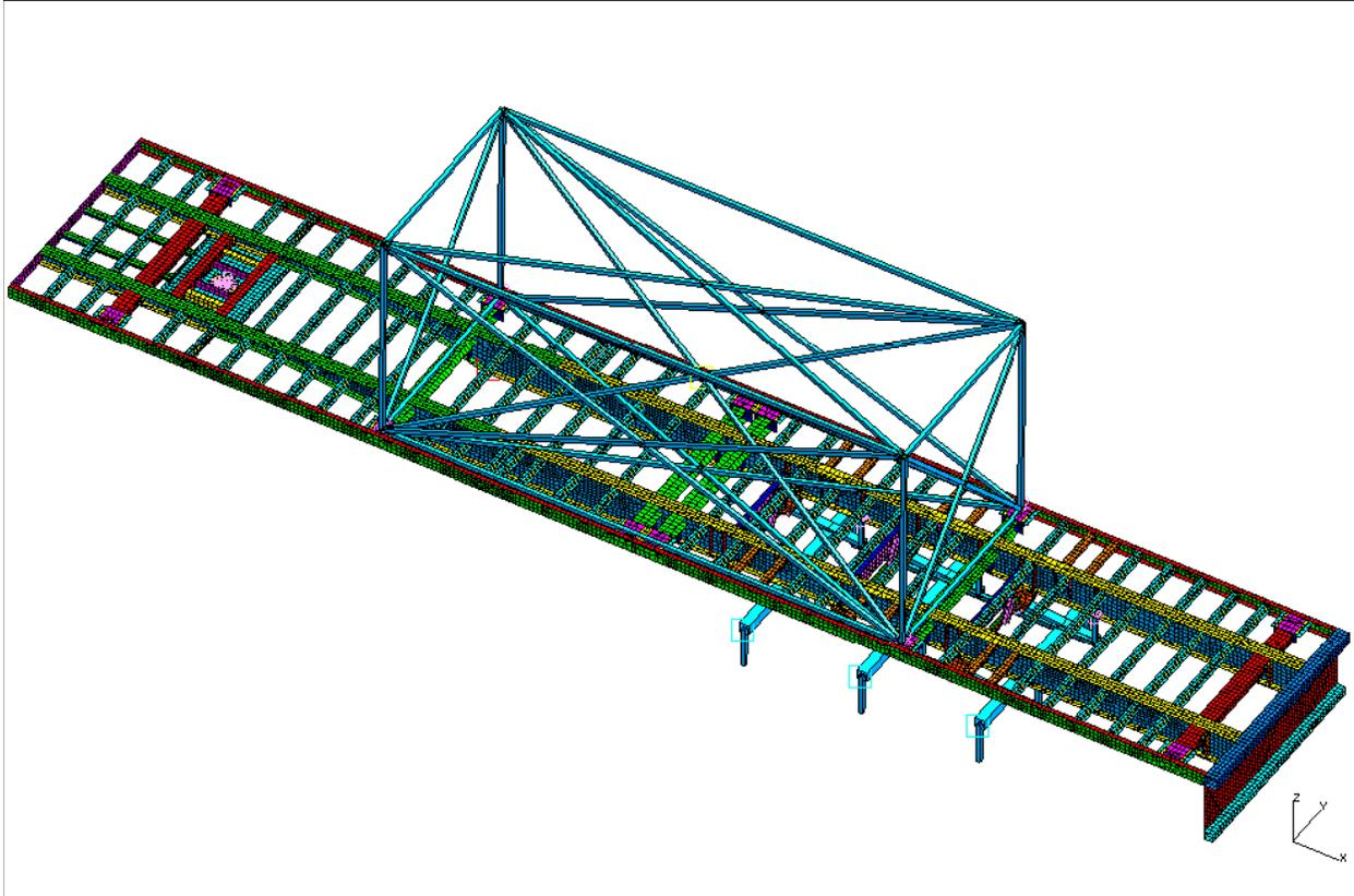
**Figure 21. FE-model of trailer case study**
