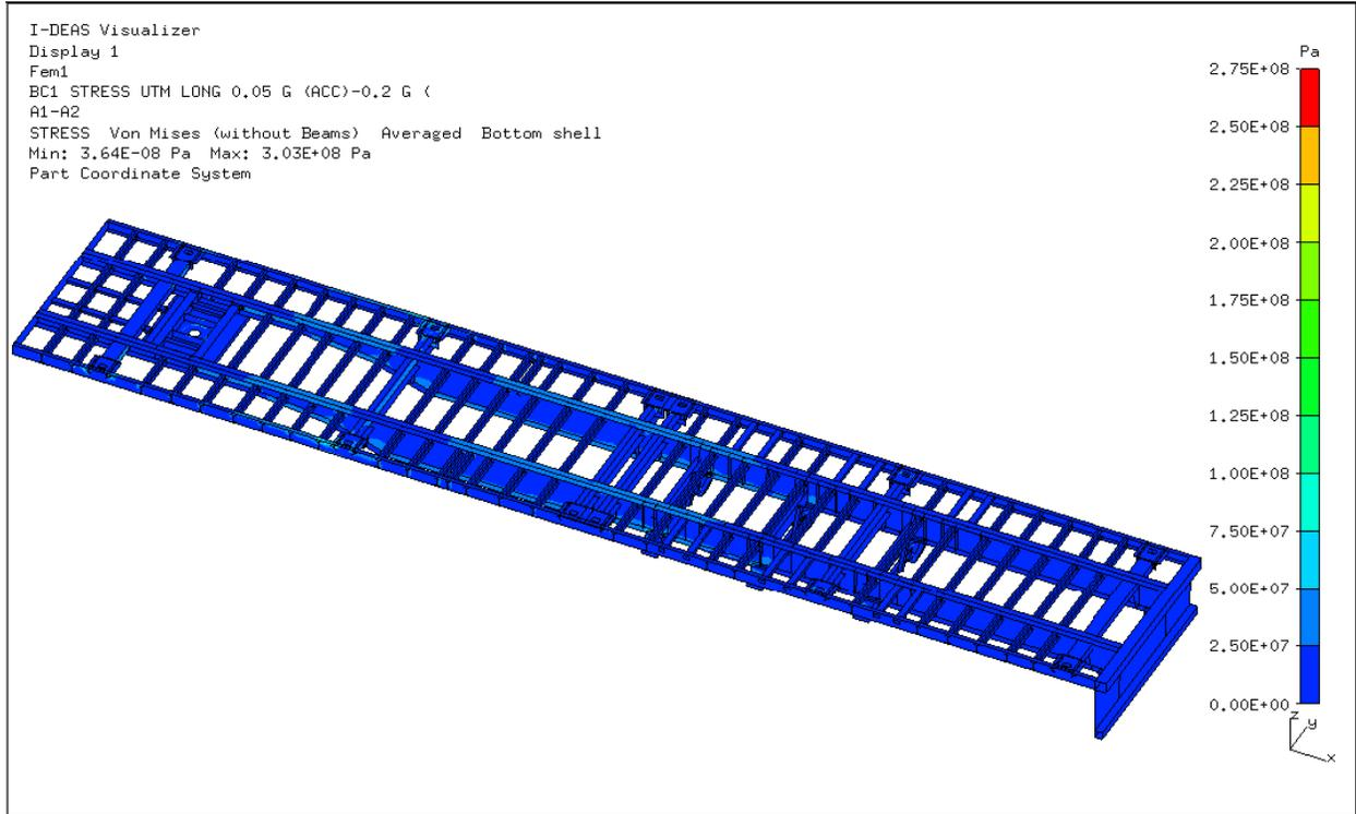
**Results (von Mises stresses in Pa) for the distributed fatigue load case.**
