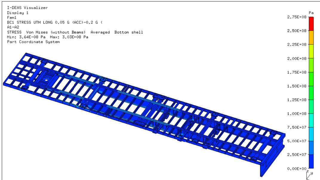
**Results (von Mises stresses in Pa) for the longitudinal fatigue load case.**
