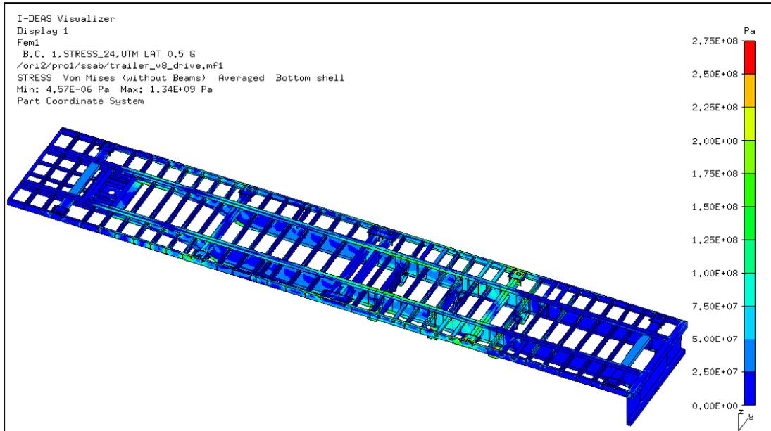
**Results (von Mises stresses in Pa) for the lateral fatigue load case.**
