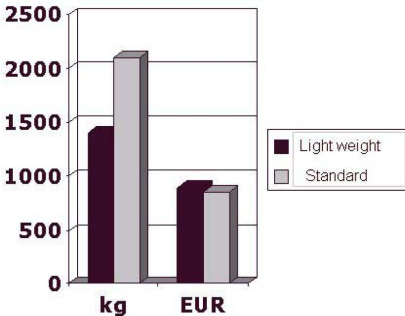
Figure 16, Comparison of weight and cost for standard trailer and a trailer in HSLA-V Steel.[2]
