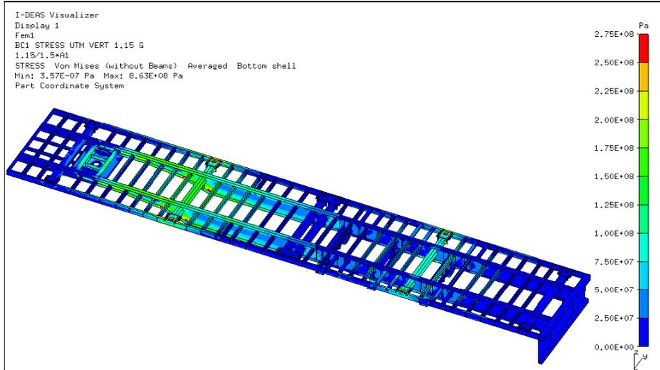
Results (von Mises stresses in Pa) for the vertical fatigue load case.
