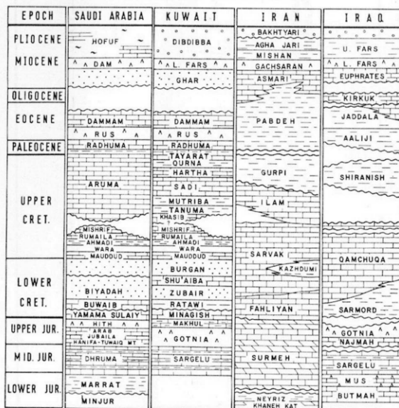
Figure 6 Some typical Middle East geological profiles (Kent, 1978).
