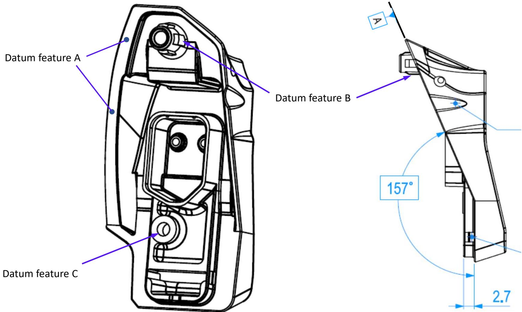
1. Both datum feature B and C are parallel but not perpendicular with primary datum feature A, I am struggling on how to build the DRF with open set up measuring. Thanks for any comments.
