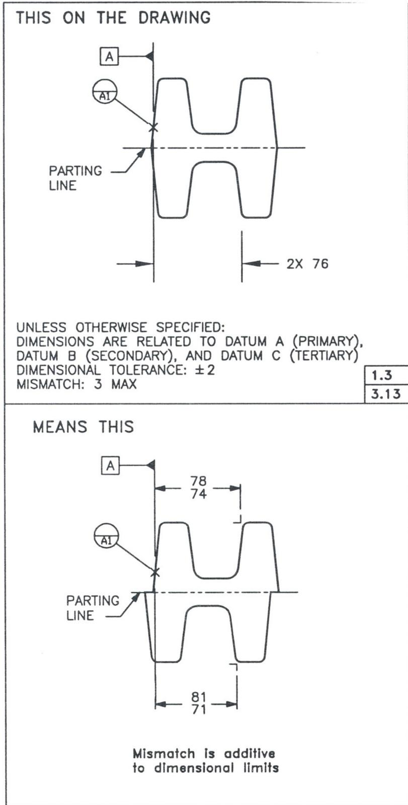
FIG. 3-8 MISMATCH TOLERANCE
