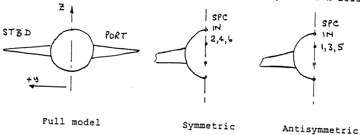
The full model loading can be split up into the components using the following formulae. It is assumed that Starboard is +ve Y.
