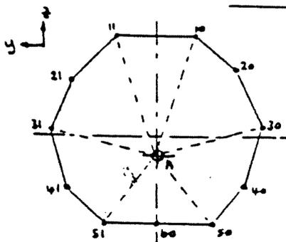
POINT A HAS ASSIGNED TO IT THE AVERAGE DISPLACEMENTS OF 6 GRID POINTS ON THE FRAME
