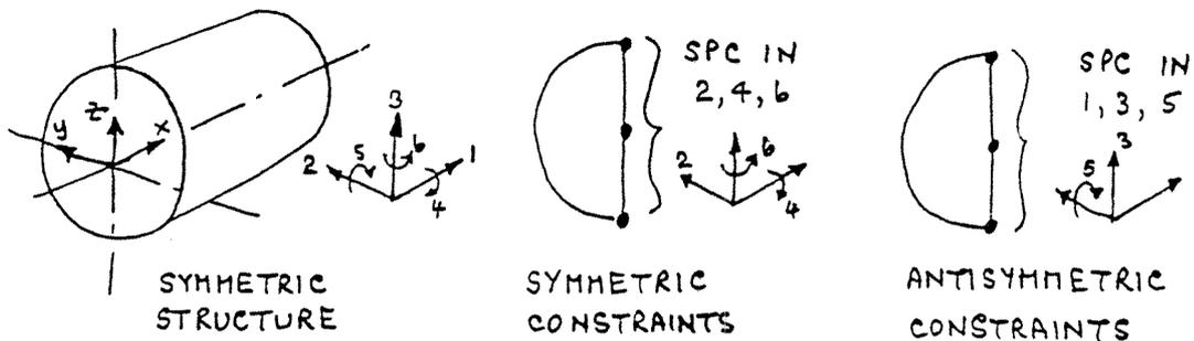
For symmetric loading the grids on the ZX plane should be constrained in the 2, 4 and 6 freedoms, i.e. preventing lateral, roll and yaw movements. For the antisymmetric case freedoms 1, 3 and 5 are constrained, preventing aft, vertical and pitch movements.
