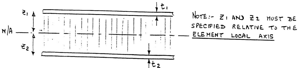
Set the PSHELL membrane thickness to  $t_1+t_2$  (if fully effective) with the associated material MID1.
