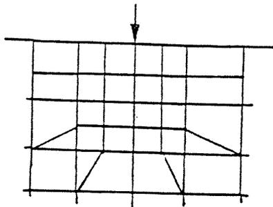
d) AVOID SOLID ELEMENTS WITH NON PARALLEL FACES FOR OUT OF PLANE CRITICAL MODELS.
