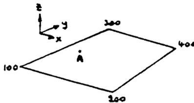
Z DISPLACEMENT OF POINT A IS THE LINEAR AVERAGE OF THE Z DISPLACEMENTS OF POINTS 100, 300 AND 400. IF POINTS 100, A AND 300 ARE COLINEAR, POINT 400 HAS NO EFFECT ON DISPLACEMENT OF A.
