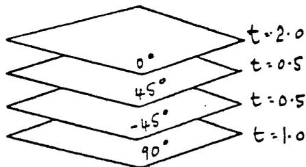
Material angles may be specified using co-ordinate systems in the F8 of the CQUAD4, or by inserting angles from edges 1-2.
