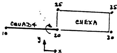
BENDING ROTATIONS FROM QUAD4 AT GRID 20 IS APPLIED TO CHEXA USING RBE1
