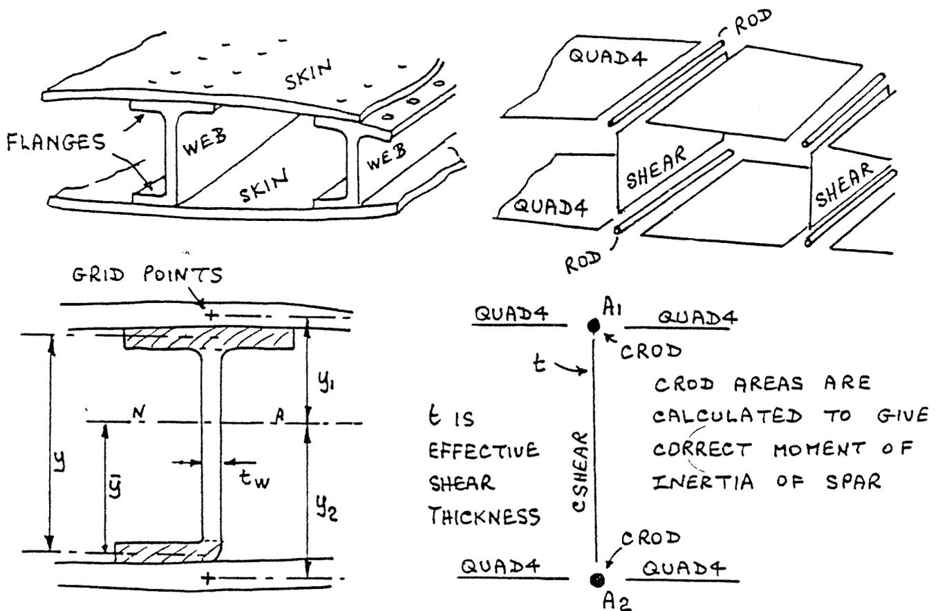
GEOMETRY IS SET UP AT SKIN MID DEPTH - QUAD4 LOADS ARE ACCURATE IF SIZES ARE CORRECT
