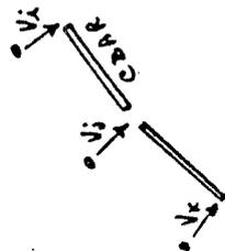
REQUIRES:- CALCULATION OF OFFSET VECTORS, SECTION PROPERTIES, ADDITIONAL ROTATIONAL D.O.F. IN MODEL.
