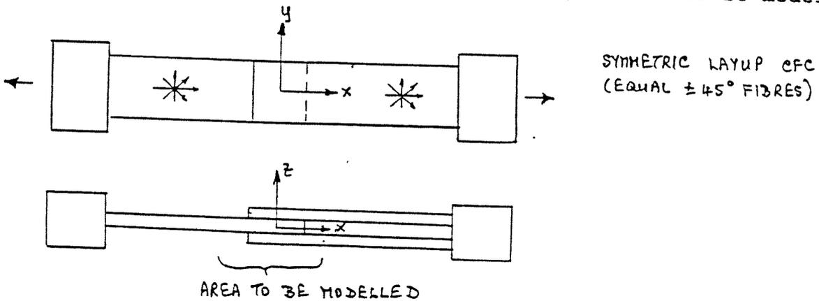
There are two planes of symmetry for SYMMETRIC conditions, XY and ZX, and the model can be reduced to 1/4 size.
