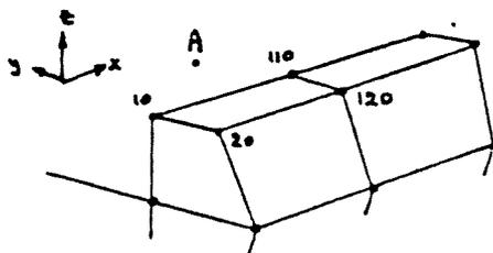
ENSURE THAT 'HARD' POINTS ARE USED WHEN INTERPOLATING FOR DISPLACEMENTS OF A.
