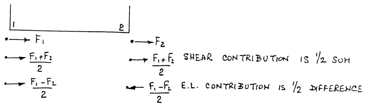
PANEL EDGE SHEAR  $q = \frac{F_1 + F_2}{l}$  WHERE  $l$  IS 1-2 LENGTH
