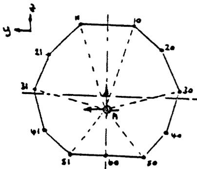
LOADS APPLIED TO POINT A WILL BE APPLIED TO THE SELECTED GRIDS IN THE USUAL 'BOLT GROUP' METHOD.
