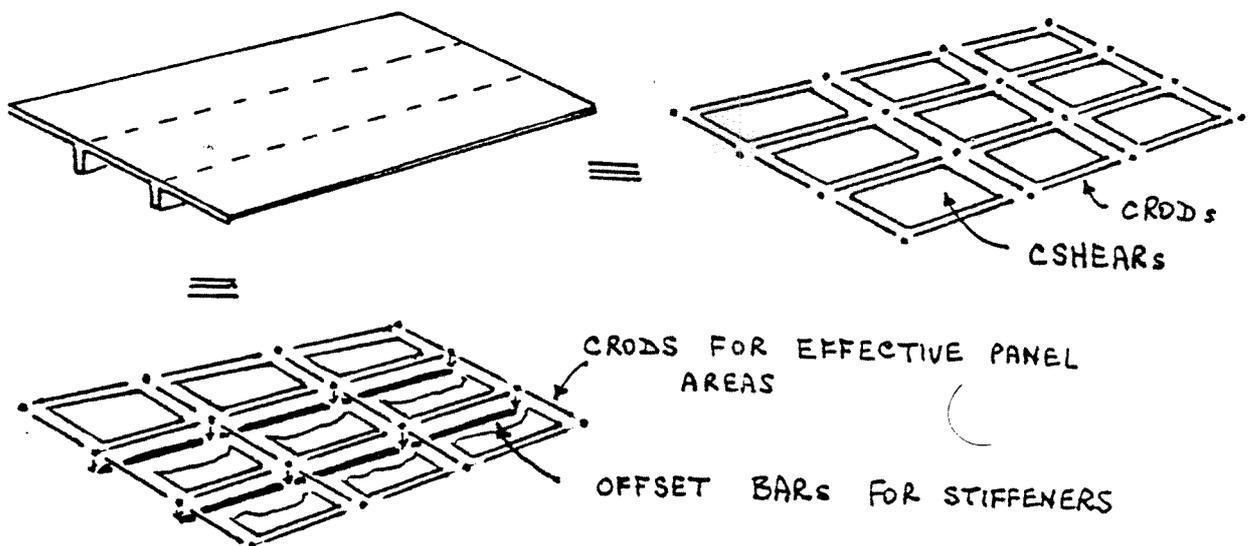
The panel effective end load areas can be set up automatically by setting F1 and F2 = 1.0 on the PSHEAR card, in which case each effective rod area will be 1/2 the panel width x thickness.
