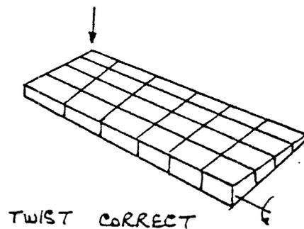
c) REFINE MESH AT HIGH LOAD POINTS
