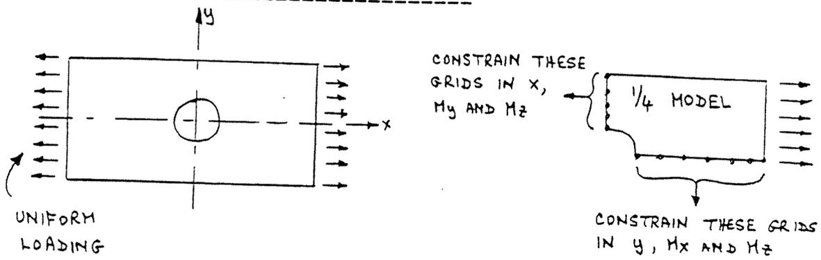
There are two planes of symmetry for SYMMETRIC conditins, ZX and YZ, and the model can be reduced to 1/4 size.
