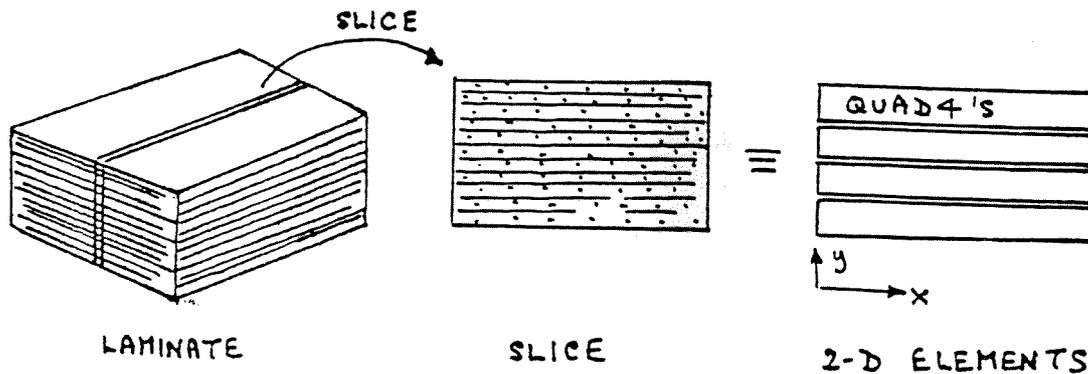
For a particular QUAD4 element the stiffness in the X direction will be dependant upon the layup stack which it represents, whilst the Y stiffness will be the glue only. Having determined  $E_x$  and  $E_y$  the usual anisotropic MAT2 data can be created by inverting the compliace (flexibility) matrix.
