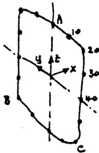
RBEl EQUATIONS LINK THE OUT-OF-PLANE FREEDOMS OF GRIDS TO THREE REFERENCE POINTS A, B AND C.
