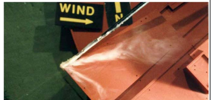
Figure 2: Corner vortices on a roof top (Photo courtesy Cermak Peterka Petersen)
