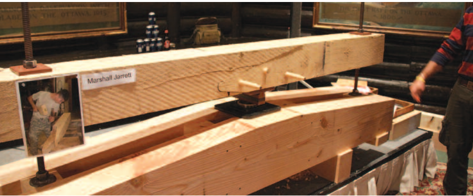
Jarrett Scarf, VMI. Code 9-VCSD. Variant on Bates. Face-halved with asymmetrical sallyed butts and three edge pegs. Moment transfer through bearing and dowel shear. Failure in tension perpendicular to the grain (minimum dowel distress).
