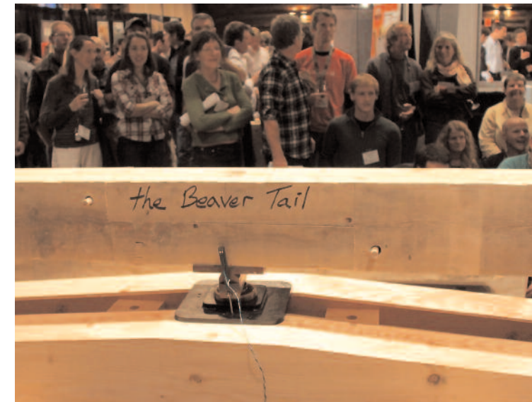
Hamlet Beaver Tail, Hamlet Heavy Timberworks. Code 14-HLMC. Edge-halved with bridled and pegged square abutments and eight face screws. Moment transfer through mechanical connectors and bearing. Failure by withdrawal of mechanical connectors and shearing of dowels. Small square brass plate is ornamental. Insert in photo at right shows shear failure of peg fastening bridled abutment.
