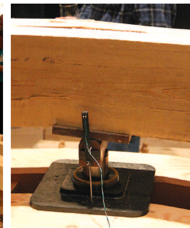
Hamlet Hemlock Solid-Sawn Beam, Hamlet Heavy Timberworks. Code 13-MN. Mother Nature's entry. Classic modulus of rupture failure, at 33,840 lbs. Test beam was parted from longer one with drill and auger bit, under desperate conditions.
