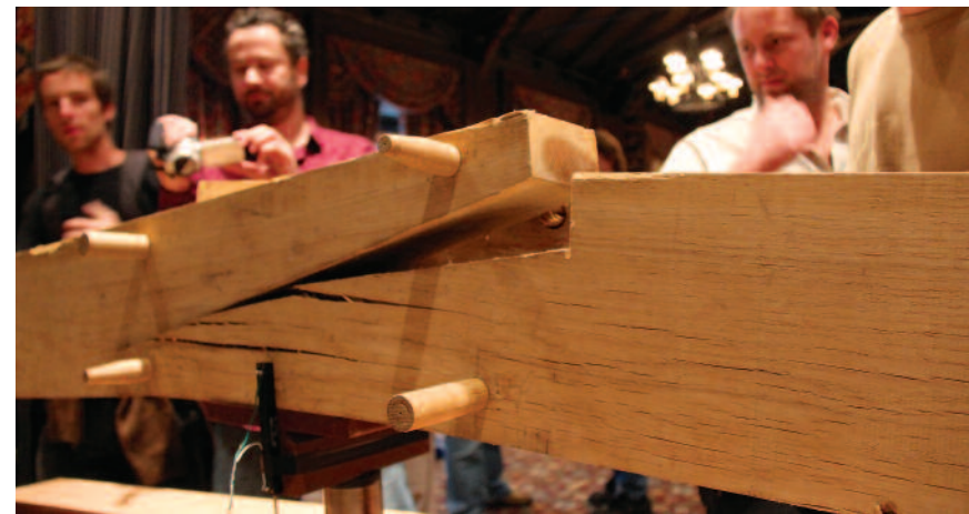
Peck Scarf, VMI. Code 10-VLSD. Face-halved scissor with four edge pegs. Moment transfer through bearing and dowel shear. Failure first through dowels followed by failure in tension perpendicular to grain.
