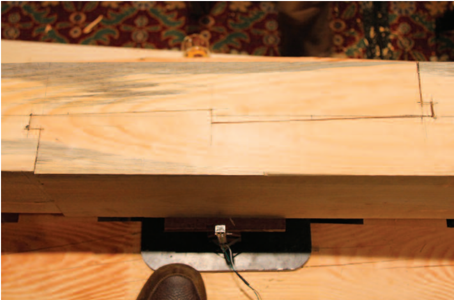
Okake Daisen, Adam Zgola. Code 15-VL. Face-halved, stop-splayed, tabled and bladed. Moment transfer through bearing alone. Block shear failure predominated with minor failure in tension perpendicular to grain. Inset shows detail of top view.
