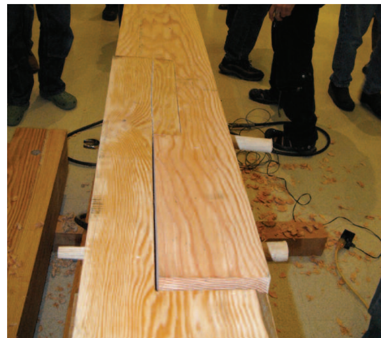
Double Deuce Scarf, Timberpeg. Code 3-VLD. Face-halved and tabled with two edge pegs. Moment transfer through bearing and dowel shear. Failure via almost pure block shear. Maker Jesse Kendall, at right, gives pep talk to scarf before testing.
