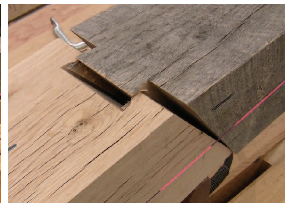
Lignatools Scarf, Stefan Richter. Code 6-BJ. Squint-butted with dovetailed bridge. Moment transfer through dovetail tenon. Failure via shear at dovetail. Joint cut impromptu at Saratoga 2009 using machine at hand.
