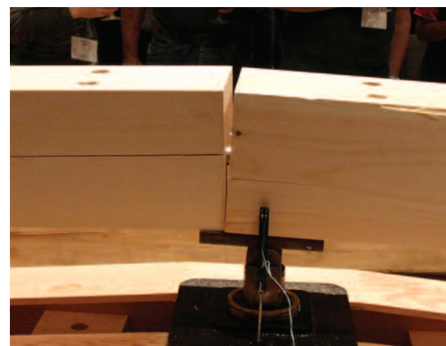
Okake Daisen, Adam Zgola. Code 15-VL. Face-halved, stop-splayed, tabled and bladed. Moment transfer through bearing alone. Block shear failure predominated with minor failure in tension perpendicular to grain. Inset shows detail of top view.
