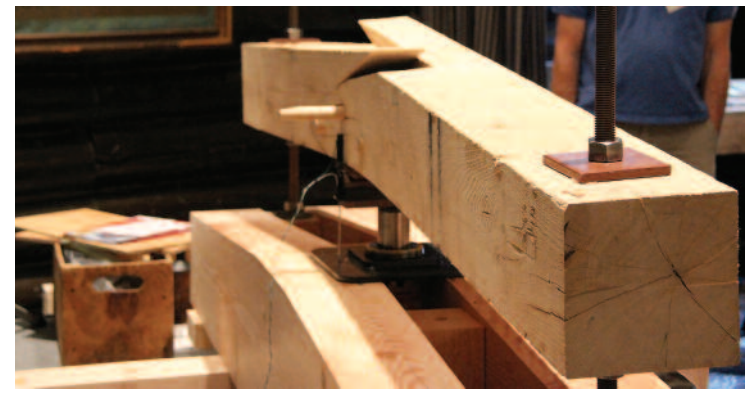
Jarrett Scarf, VMI. Code 9-VCSD. Variant on Bates. Face-halved with asymmetrical sallyed butts and three edge pegs. Moment transfer through bearing and dowel shear. Failure in tension perpendicular to the grain (minimum dowel distress).
