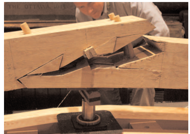
Peck Scarf, VMI. Code 10-VLSD. Face-halved scissor with four edge pegs. Moment transfer through bearing and dowel shear. Failure first through dowels followed by failure in tension perpendicular to grain.
