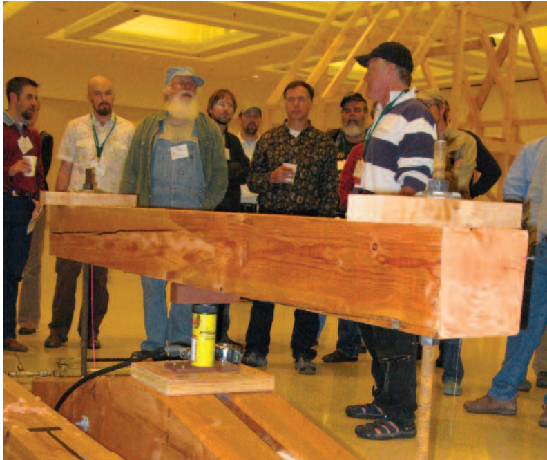
SOB (Saratoga or Bust) Scarf, Loyalist Timberframes. Code 2-VCS. Face-halved with sallyed and bridled butts. Moment transfer through bearing. Tension perpendicular to the grain failure as load pried joint apart.
