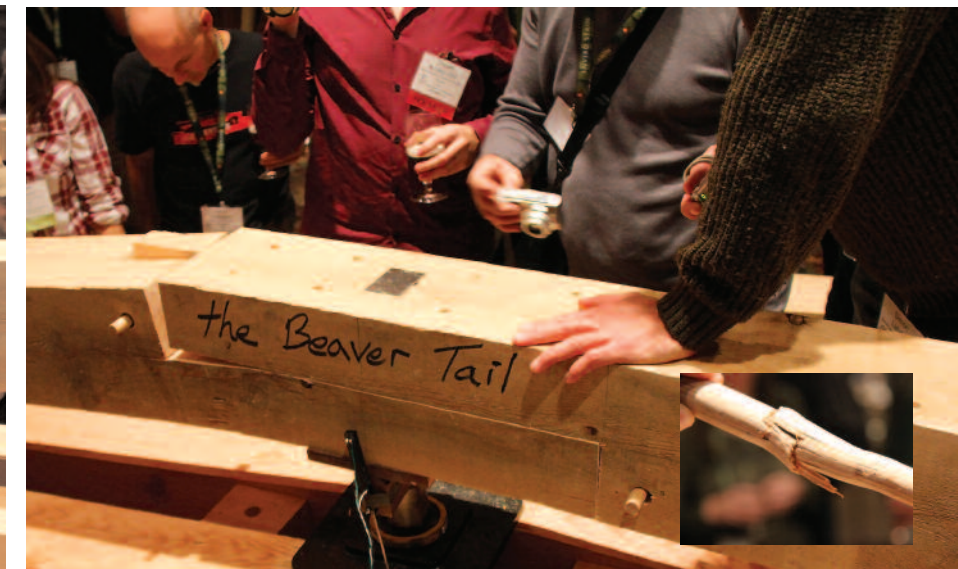
Hamlet Beaver Tail, Hamlet Heavy Timberworks. Code 14-HLMC. Edge-halved with bridled and pegged square abutments and eight face screws. Moment transfer through mechanical connectors and bearing. Failure by withdrawal of mechanical connectors and shearing of dowels. Small square brass plate is ornamental. Insert in photo at right shows shear failure of peg fastening bridled abutment.
