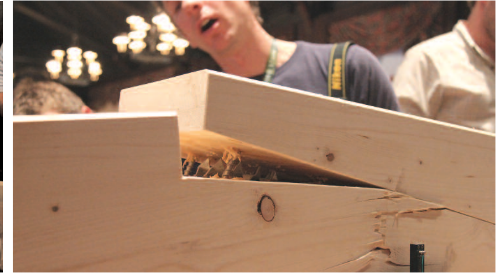
Heco Scarf, Herrmann's Timber Frame Homes. Code 12-HLMC. Edge-halved and stop-splayed with numerous face screws. Moment transfer through axial loading of screws. Failure by withdrawal of screws and breaking of glulam fingerjoint. Toothed connector inside was ineffectual.
