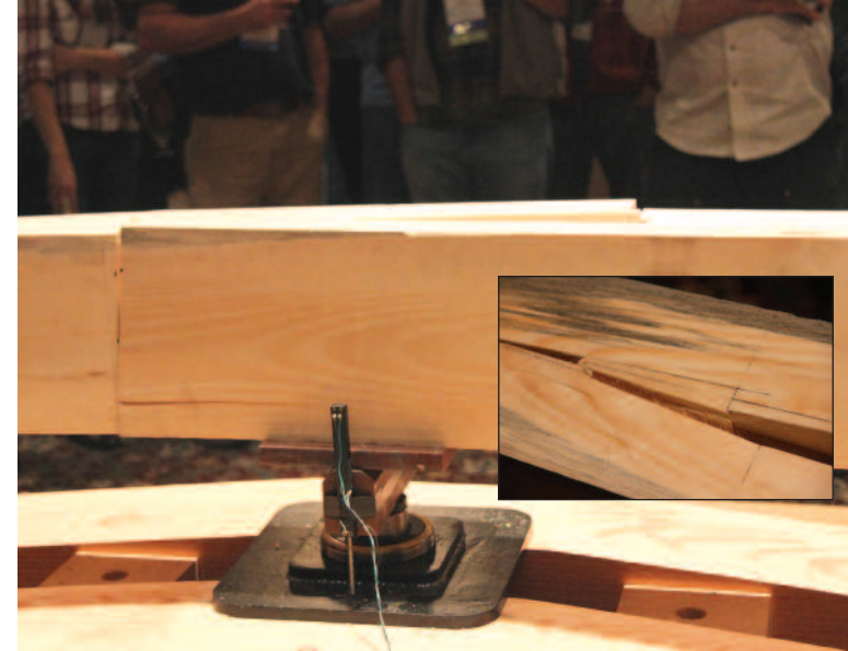
Okake Daisen, Adam Zgola. Code 15-VL. Face-halved, stop-splayed, tabled and bladed. Moment transfer through bearing alone. Block shear failure predominated with minor failure in tension perpendicular to grain. Inset shows detail of top view.
