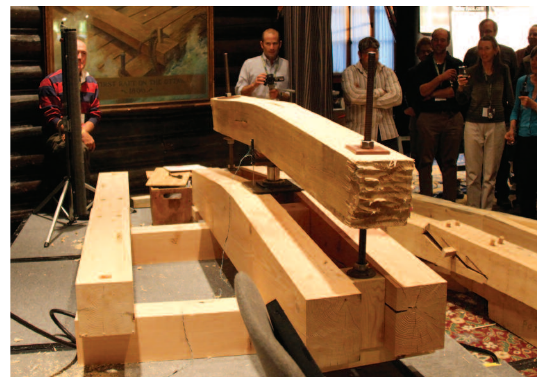
Hamlet Hemlock Solid-Sawn Beam, Hamlet Heavy Timberworks. Code 13-MN. Mother Nature's entry. Classic modulus of rupture failure, at 33,840 lbs. Test beam was parted from longer one with drill and auger bit, under desperate conditions.
