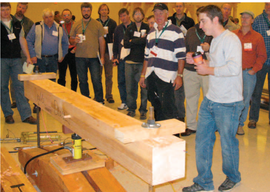
Double Deuce Scarf, Timberpeg. Code 3-VLD. Face-halved and tabled with two edge pegs. Moment transfer through bearing and dowel shear. Failure via almost pure block shear. Maker Jesse Kendall, at right, gives pep talk to scarf before testing.
