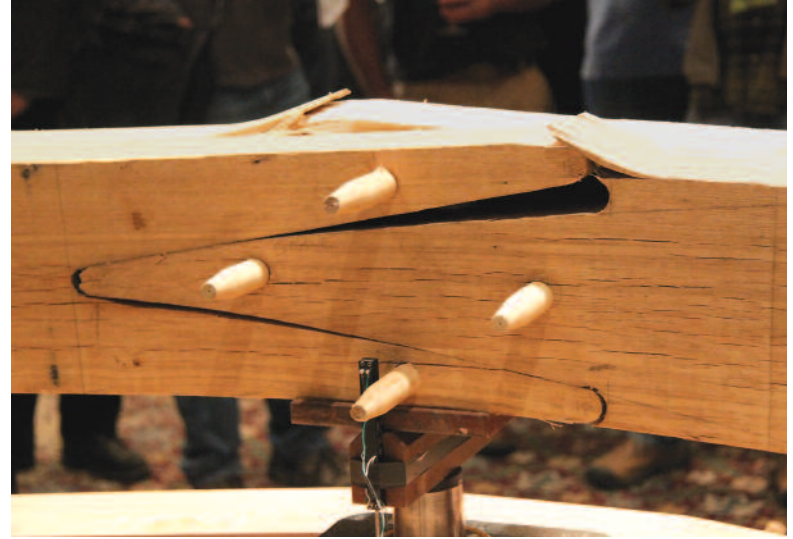
Bates Scarf, Virginia Military Institute (VMI). Code 8-VCSD. Face-halved with sallyed butts and four edge pegs. Moment transfer in bearing and dowel shear. Failure in tension perpendicular to grain and dowel shear.
