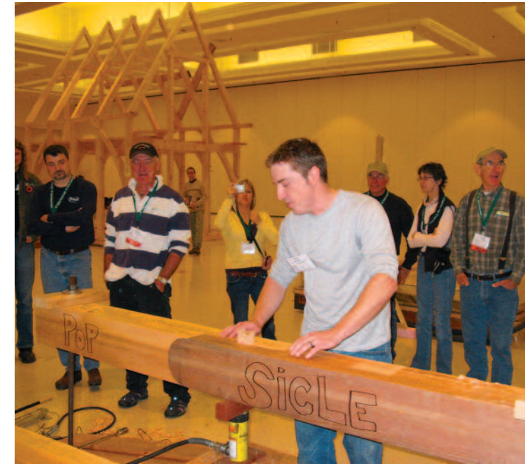
Pop-Sicle Scarf, Timberpeg. Code 5-VLW. Face-halved and keyed with radiused butts. Moment transfer primarily through bearing. Failures via tension perpendicular to grain and key shear. Insert in photo at right shows failure of folding-wedged key.
