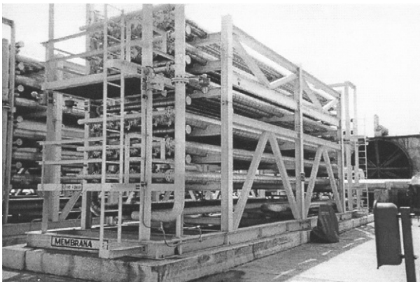
FIGURE 1-16 Horizontal membrane skid.
