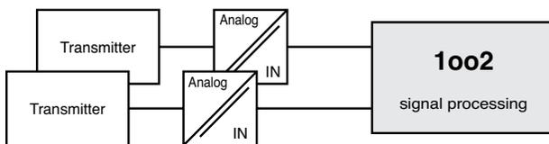
**Hardware fault tolerance:** as a rule 1oo2 is necessary
