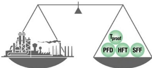
In all risk-reducing measures, it is the overall result that is critical. Thus, it is not possible to consider an individual device in the signal circuit without reference to the remaining components. Furthermore, the evaluation structure and the organizational measures, such as the interval between repeated function tests must also be considered.
