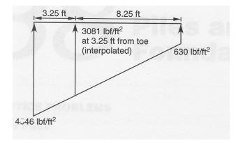
The shearing force is found by multiplying the total upward normal force and the coefficient of shearing (internal) friction.
