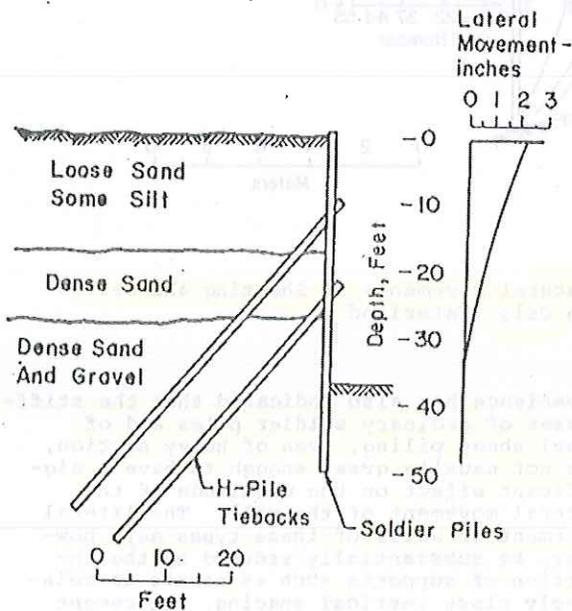
Fig. 16. Section through Cut in Sand Supported by Tieback System; Lateral Movement of Soldier-Pile Wall during Excavation
