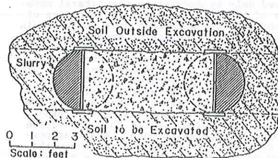
Fig. 29. Horizontal Section through Typical SPTC Wall
