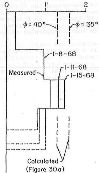
Fig. 34. Strut Loads in Cut in Dense Clayey Sands and Stiff Sandy Clays in Oakland, California
