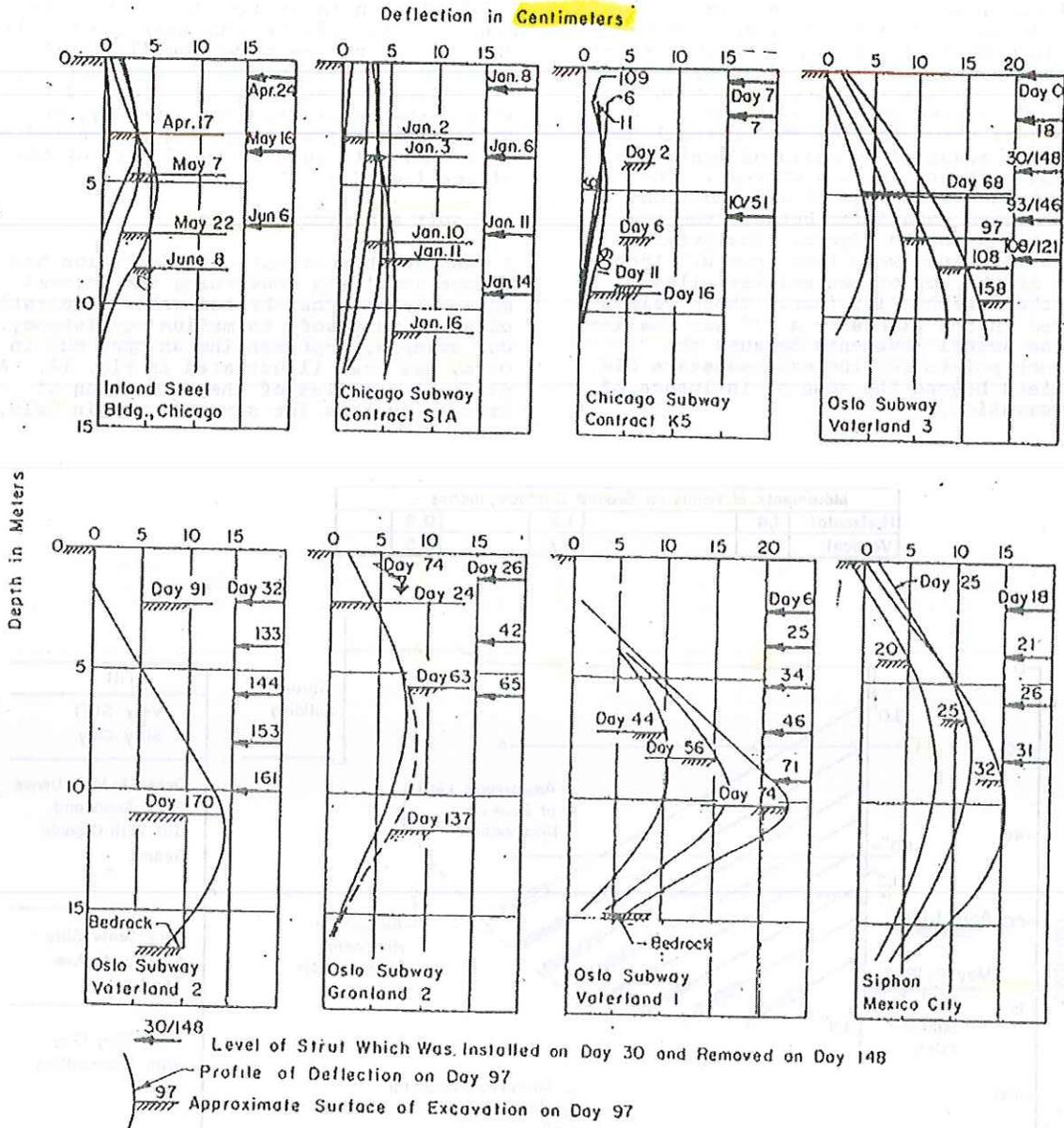
Fig. 19. Profiles of Deflections of Soldier-Pile and Sheet-Pile Walls of Various Open Cuts in Plastic Clays of Very Soft to Medium Consistency
