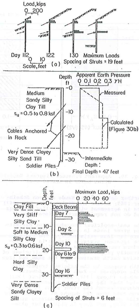
Fig. 31. Loads in Bracing Systems of Several Cuts in Clays. (a) Horizontal Components of Loads in Inclined Bracing of a Cut in St. Louis, Illustrated in Fig. 21; (b) Apparent Pressure Diagrams from Forces Measured in Tiebacks at Pickering Generating Station, Ontario; (c) Preliminary Values of Forces in Struts, Contract K5, Chicago
