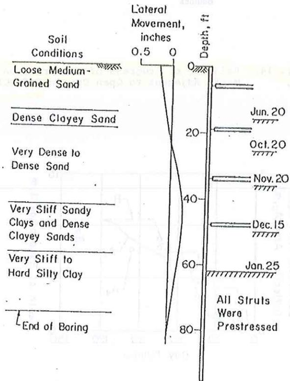
Fig. 17. Section through Cut in Dense Cohesive Sands and Stiff Silty or Sandy Clays, Supported by Cross-Lot Bracing, in Oakland, California; Lateral Movement of Soldier-Pile Wall during Excavation
