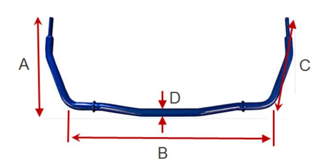
Figure 1: basic sway bar dimensions
