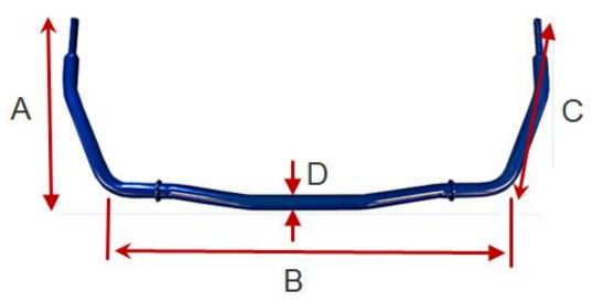
Deflection from Torsion  $(\delta_t)$  Deflection from Bending  $(\delta_b)$ These deflections are the deflections of the ends (at endlink location) Angular Deflection of Arm  $(\theta_t)$  - measured in radians for small angles  $\theta_t \equiv \frac{\delta_t}{A}$
