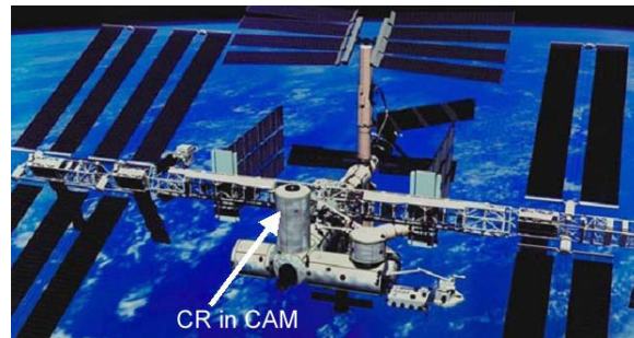
FIGURE K-6. Shows International Space Station with Centrifuge Accommodation Module (CAM). The Centrifuge Rotor (CR) is at the Arrow Location in the CAM [4]
