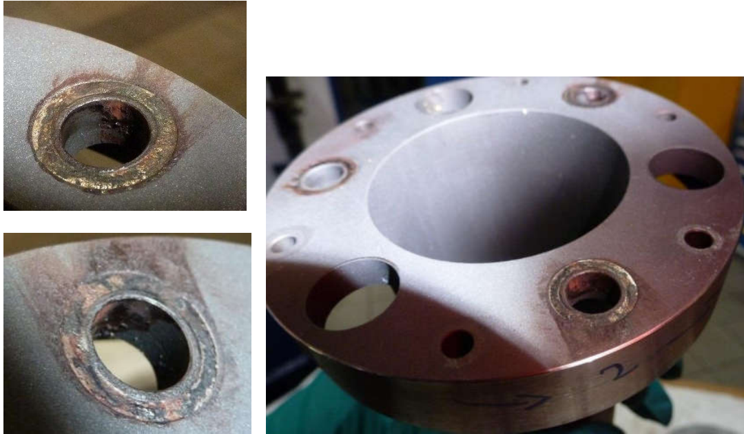
Figure 5 - Spacer HPC side condition with damage around the bolt holes
