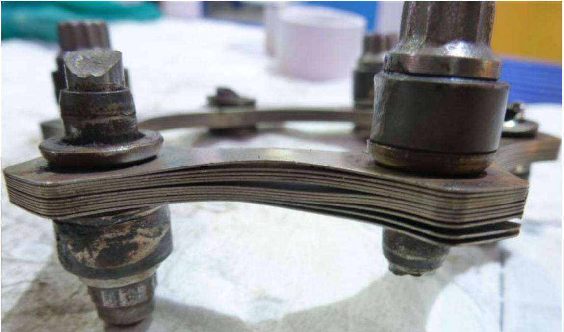
Figure 11 - LPC membrane pack with wear damage on overload collars
