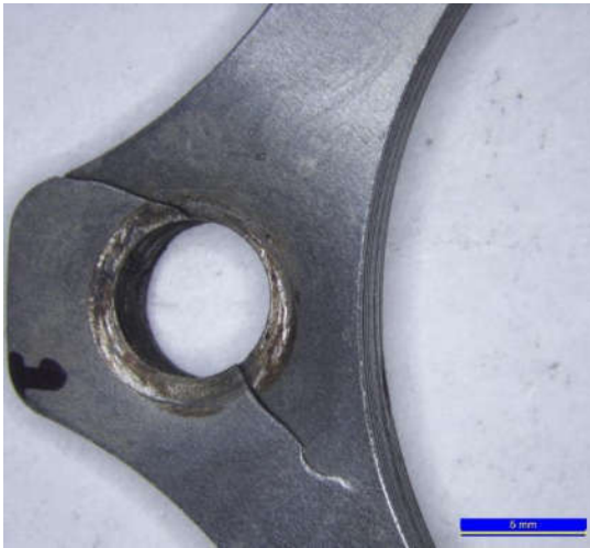
Figure 10 - membrane hole with fretting damage around the hole and crack propagating from the bolt hole and failure across of the membranes
