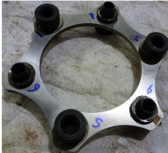
Figure 3 - membrane pack showing fretting residue around the membrane pack but with an overall good condition and no noticeable bowing
