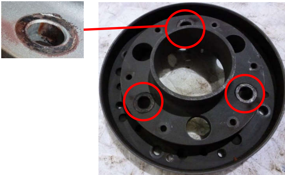
Figure 4 - Guard ring showing signs of wear around the bolt hole washers which grooved the surface
