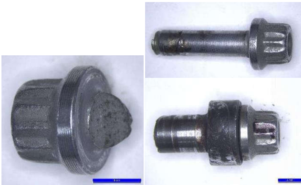
Figure 14 - Failed bolts, highlighting the location of failure i.e. fillet radius (left), threads (middle) and shank (right)
