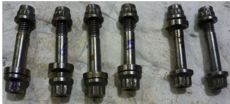
Figure 6 - HPC side bolts with an overall good condition with minor fretting on some of the bolts shank
