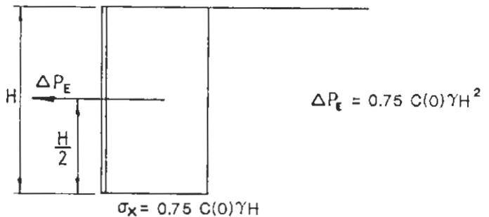
FIG. 3.4 EQ PRESSURE INCREMENT ON STIFF WALL
