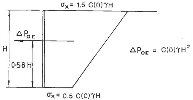
FIG. 3.3 EQ PRESSURE INCREMENT ON RIGID WALL
