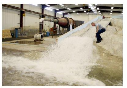
In this Friday, June 16, 2017, photo, hydraulic engineering professor Michael Johnson looks at the water flow on a replica of the Oroville Dam spillway at Utah State University's Water Research Laboratory, in Logan, Utah. California water officials are relying on key hydrology tests being performed on the replica of the spillway to pinpoint what repairs will work best at the tallest dam in the U.S for a spillway that was torn apart in February. (AP Photo/Rick Bowmer)
