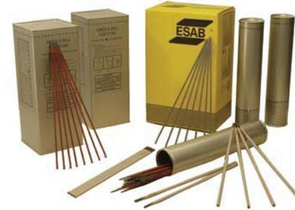
Atom Arc 9018-B9 is designed to weld the modified 9% Cr - 1% Mo steels known by the designations T91, P91 or Grade 91. These steels are designed to provide improved creep strength, toughness, fatigue and oxidation, and corrosion resistance at elevated temperatures.
